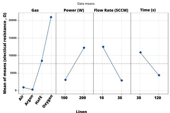
Fig. 13 Linen main effects plot demonstrating linen's sensitivity to all plasma parameters under test.
