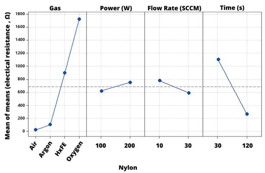
Fig. 8 Main effects plot of MC-Nylon demonstrating the large effects of gas type and treatment time, and more neglible effects of power and flow rate.
