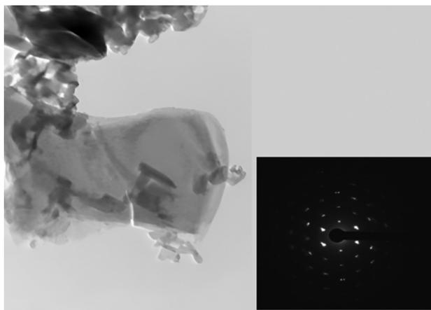
Fig. 4 TEM micrograph of MXene  $\text{Ti}_3\text{C}_2$  powder. Inset, corresponding diffraction pattern, indicating single layer MXene formation.
