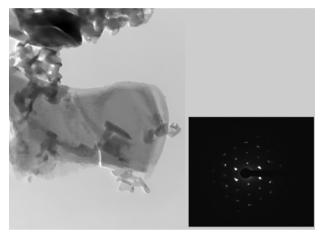
Fig. 4 TEM micrograph of MXene Ti<sub>3</sub>C<sub>2</sub> powder. Inset, corresponding diffraction pattern, indicating single layer MXene formation.
