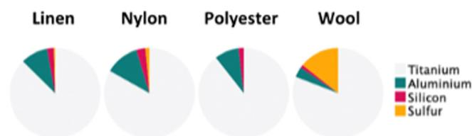
Fig. 2 Inorganic elemental composition main components (XRF data) showing Ti content that confirms successful MXene coating, but presence of Al indicates unetched MAX phase.
