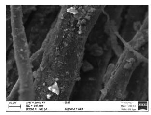
Fig. 5 MXene coating on linen pre-treated by argon gas (200 W, 30 SCCM, 120 s) showing MXene flakes adhered across the surface.
