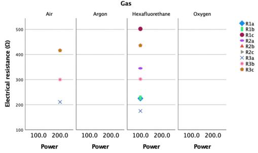
Fig. 10  $\Omega$  of MC-wool by gas type and power up to 500  $\Omega$  demonstrating the strong effect of HxFE low power treatment, and highlighting the negligible effects of other treatment parameters.
