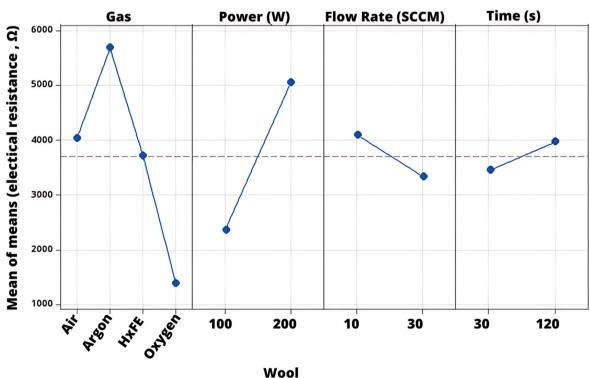
Fig. 9 Main effects plot of MC-wool demonstrating the significant effects of gas type and power on the  $\Omega$ .
