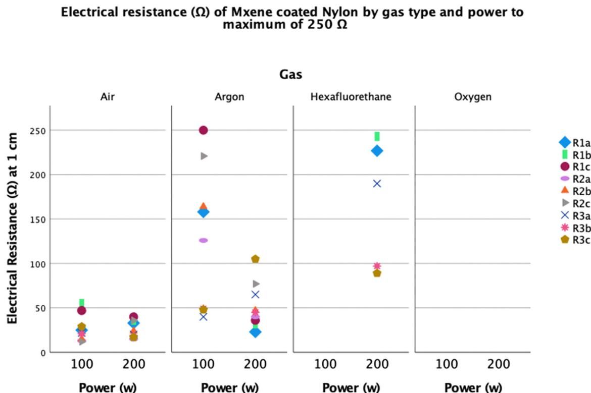
Fig. 7 Electrical resistance of MC-Nylon by gas and power parameters up to 250  $\Omega$ , demonstrating the consistently excellent results of air treated MC-Nylon and the consistently poor results of oxygen treated MC-Nylon.
