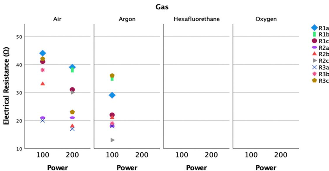
Fig. 12  $\Omega$  of MC-polyester by gas type and power to 50  $\Omega$ . The results here highlight that although the main effects overall are not significantly responsive to power, there are interactions which are not detected. MC-polyester's  $\Omega$  is lower under argon with low power treatment than with argon under high power treatment.
