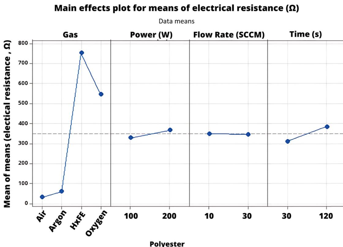
Fig. 11 Polyester main effects plot showing the significant effect of gas type and negligible effects of other parameters.
