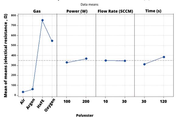
Fig. 11 Polyester main effects plot showing the significant effect of gas type and negligible effects of other parameters.
