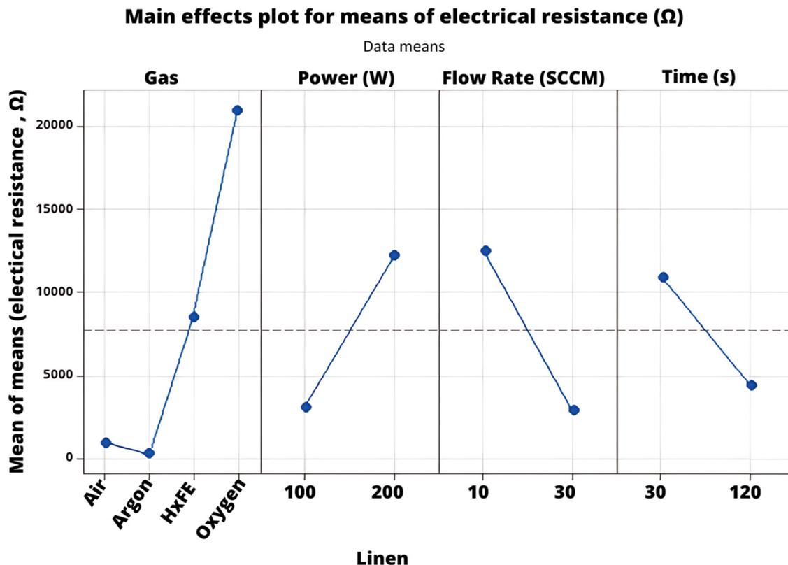
Fig. 13 Linen main effects plot demonstrating linen's sensitivity to all plasma parameters under test.
