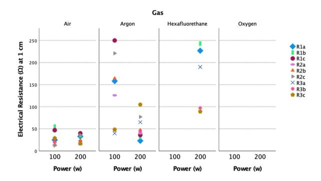
Fig. 7 Electrical resistance of MC-Nylon by gas and power parameters up to 250  $\Omega$ , demonstrating the consistently excellent results of air treated MC-Nylon and the consistently poor results of oxygen treated MC-Nylon.
