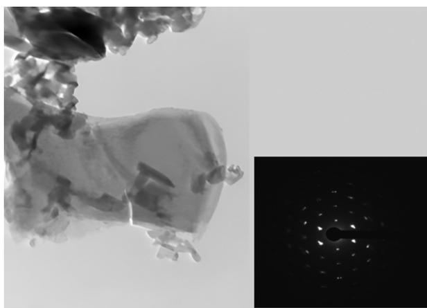
Fig. 4 TEM micrograph of MXene  $Ti_3C_2$  powder. Inset, corresponding diffraction pattern, indicating single layer MXene formation.
