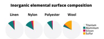
Fig. 2 Inorganic elemental composition main components (XRF data) showing Ti content that confirms successful MXene coating, but presence of Al indicates unetched MAX phase.
