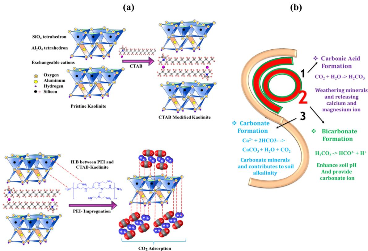
Fig. 1 (a) Synthesis of PEI-impregnated clay-based CO<sub>2</sub>-enriched fertilizers, and (b) illustration of possible interactions of CO<sub>2</sub> in soil.
