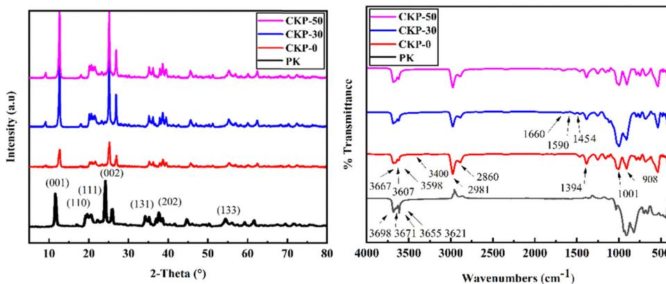
Fig. 7 FTIR and XRD analysis of all prepared fertilizers after the CO<sub>2</sub> adsorption study.
