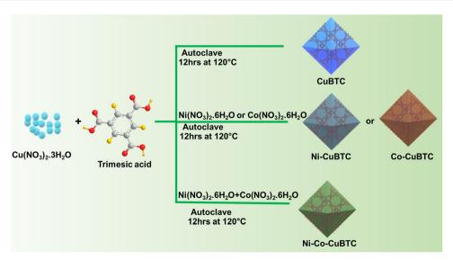
Scheme 1 Synthesis process diagram for CuBTC, Ni-CuBTC, Co-CuBTC, and Co-Ni-CuBTC
