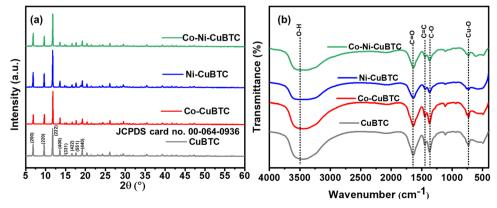
Fig. 1 (a) PXRD patterns, and (b) FTIR spectra of CuBTC, Ni-CuBTC, Co-CuBTC and Co-Ni-CuBTC
