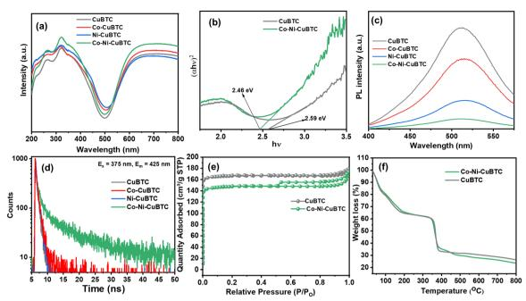
Fig. 4 (a) UV-DRS plots, (b) Tauc plots, (c) PL spectra, (d) TCSPC analysis, (e) N2 adsorption-desorption isotherm, and (f) TGA plots of the prepared composites.
