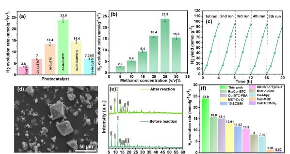
Fig. 5 (a) Histogram showing PHE rates of synthesised photocatalysts, (b) PHE rates of Co-Ni-CuBTC at various methanol concentrations, (c) stability test of the optimised catalyst (Co-Ni-CuBTC), (d) SEM images, (e) PXRD pattern of Co-Ni-CuBTC before and after the photocatalytic reaction, and (f) Comparison of PHE rates between Co-Ni-CuBTC and CuBTC-based photocatalysts.
