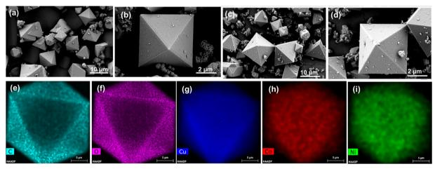
FESEM images of (a) and (b) CuBTC, (c) and (d) Co-Ni-CuBTC. HAADF-STEM images of Co-Ni-CuBTC (e) C, (f) O, (g) Cu, (h) Co, and (i) Ni.
