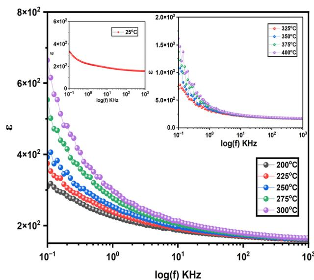
Fig. 5 Frequency-dependent dielectric constant ( $\epsilon_r$ ) at different temperatures.
