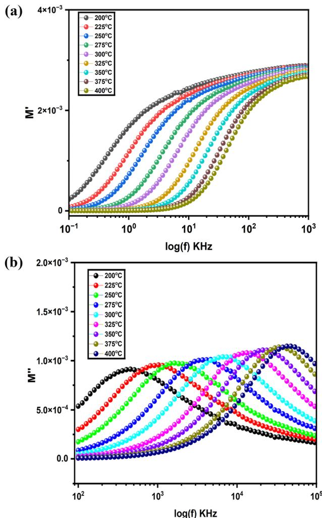
Fig. 8 (a) Frequency-dependent variation of  $M'$  at different temperatures. (b) Frequency-dependent variation of  $M''$  at different temperatures.
