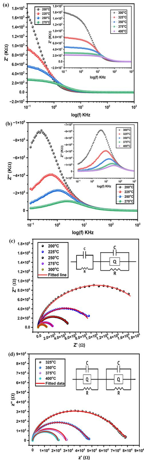
Fig. 7 (a) Variation of  $Z'$  with frequency at different temperatures. (b) Variation of  $Z''$  with frequency at different temperatures. (c) Variation of  $Z''$  with  $Z'$  (Nyquist plot) at selected temperatures. (d) Variation of  $Z''$  with  $Z'$  (Nyquist plot) at selected temperatures.
