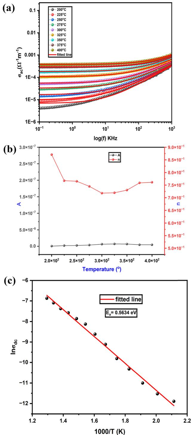
Fig. 9 (a) Variation of ac conductivity with frequency at selected temperatures fitted with Jonscher's power law. (b) Variation of  $A$  and  $n$  with temperature. (c) Variation of dc conductivity with inverse of temperature.
