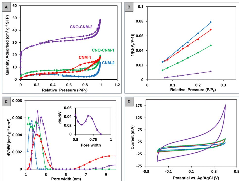
Fig. 6 (A)  $N_2$  adsorption–desorption isotherms of the synthesized materials with corresponding (B) BET curves and (C) differential pore size distributions based on DFT calculations. (D) CV curves of GCE electrodes modified with the synthesized materials recorded in 1 M KOH at a scan rate of  $50 \text{ mV s}^{-1}$ .
