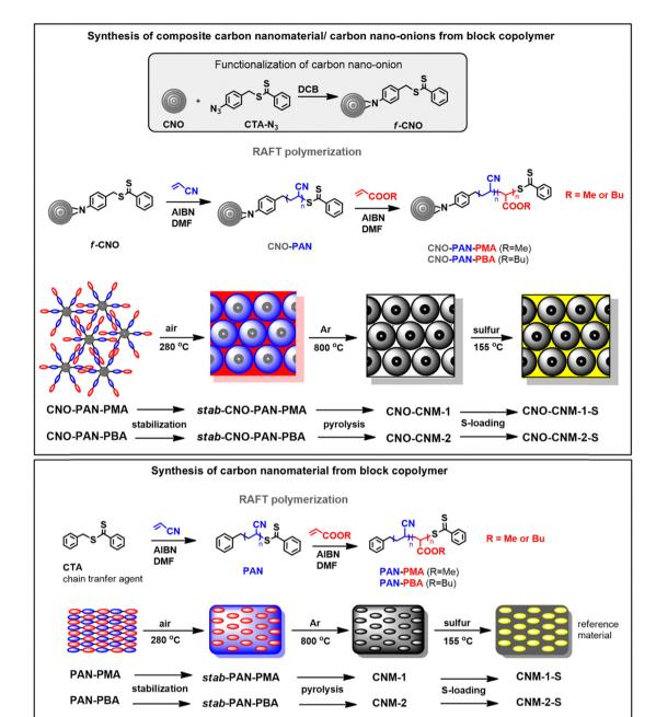
Fig. 1 Schematic representation of the synthesis of CNM-1-S and CNM-1-S and their hybrids with CNOs (CNO-CNM-1-S and CNO-CNM-1-S).
