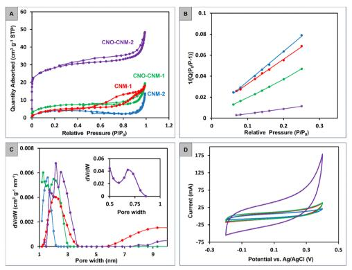
Fig. 6 (A) N<sub>2</sub> adsorption – desorption isotherms of the synthesized materials with corresponding (B) BET curves and (C) differential pore size distributions based on DFT calculations. (D) CV curves of GCE electrodes modified with the synthesized materials recorded in 1 M KOH at a scan rate of 50 mV s<sup>-1</sup>.
