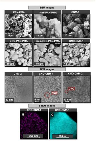
Fig. 5 SEM of CNM-1 and CNO-CNM-1 before and after thermal treatment, HRTEM of carbon nanomaterials, and STEM-EDX elemental map of CNO-CNM-1.
