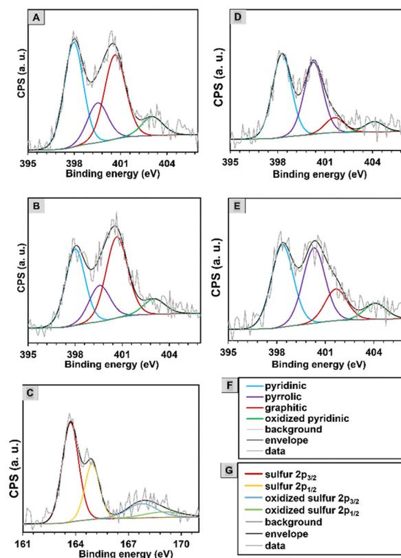
Fig. 4 XPS spectra of the N 1s spectral region of (A) **CNM-1** and (B) **CNO-CNM-1**, S 2p spectral regions of (C) **CNM-S-2**, N 1s spectral region of (D) **CNM-2** and (E) **CNM-S-2**, (F) legend of nitrogen spectra, and (G) legend of the sulfur spectrum.
