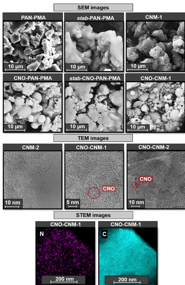
Fig. 5 SEM of CNM-1 and CNO-CN1 before and after thermal treatment, HRTEM of carbon nanomaterials, and STEM-EDX elemental map of CNO-CN1.
