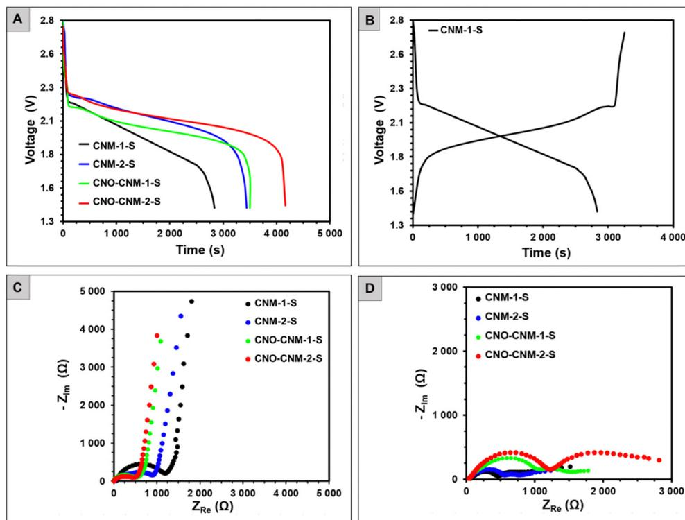
Fig. 7 Discharge curves of the Li–S batteries with four different cathode materials (A) with an example of charge/discharge profiles for CNM-1-S cathode (B) recorded at the rate of  $C/20$ . Nyquist plots of the Li–S batteries with four different cathode materials after the cell assembly (C) and after the first charging process (D) the electrolyte was 1 M LiTFSa in DOL/DME (1 : 1 v/v).
