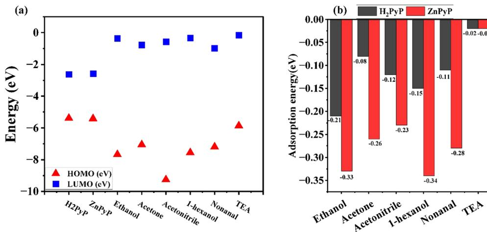
Fig. 9 (a) HOMO–LUMO values of H<sub>2</sub>PyP, ZnPyP and VOCs. (b) Adsorption energy of VOCs with H<sub>2</sub>PyP and ZnPyP.
