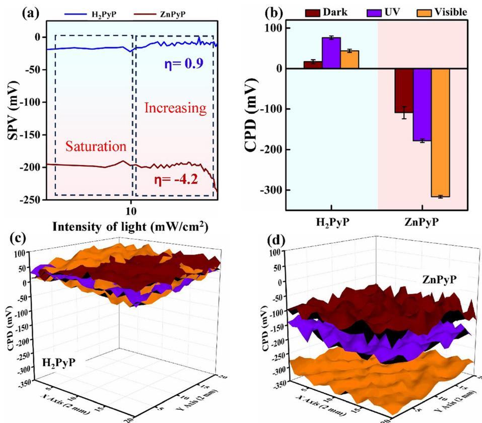
Fig. 4 (a) Surface photovoltage changes of H<sub>2</sub>PyP and ZnPyP in air. (b) CPD changes from dark to UV and visible light illumination in H<sub>2</sub>PyP and ZnPyP. 3D raster scan images under dark, UV and visible light illumination in (c) H<sub>2</sub>PyP and (d) ZnPyP under ambient air.
