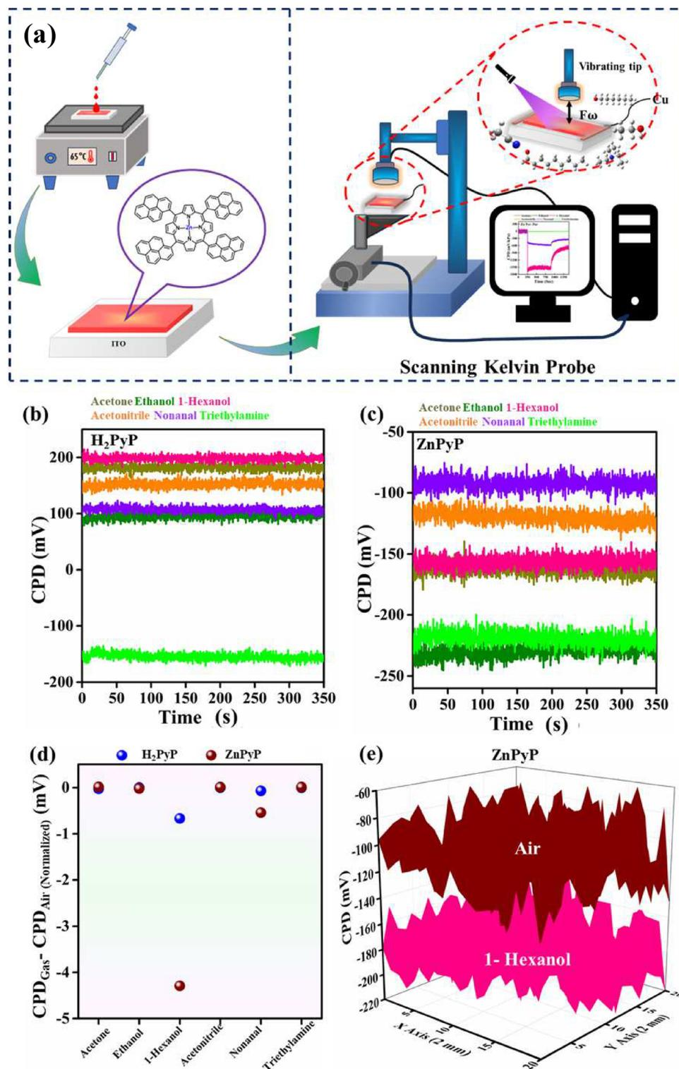
Fig. 3 (a) Schematic of the SKP device used in the present work. Time evolution of the CPD signal under exposure to various VOCs in the dark for (b) H<sub>2</sub>PyP and (c) ZnPyP. (d) Normalized CPD plots for VOCs with respect to air for the samples. (e) 3D raster scan image under ambient air and 1-hexanol for ZnPyP.
