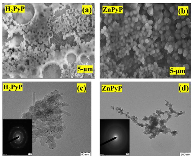
Fig. 2 HR-SEM images of (a) H<sub>2</sub>PyP and (b) ZnPyP; high-resolution transmittance electron microscopy images of H<sub>2</sub>PyP (c) showing the overall picture of the agglomerated structure, with the inset showing the SAED pattern of polycrystalline H<sub>2</sub>PyP; and (d) ZnPyP showing the agglomerated carbon layer, with the inset showing the SAED pattern of amorphous ZnPyP.
