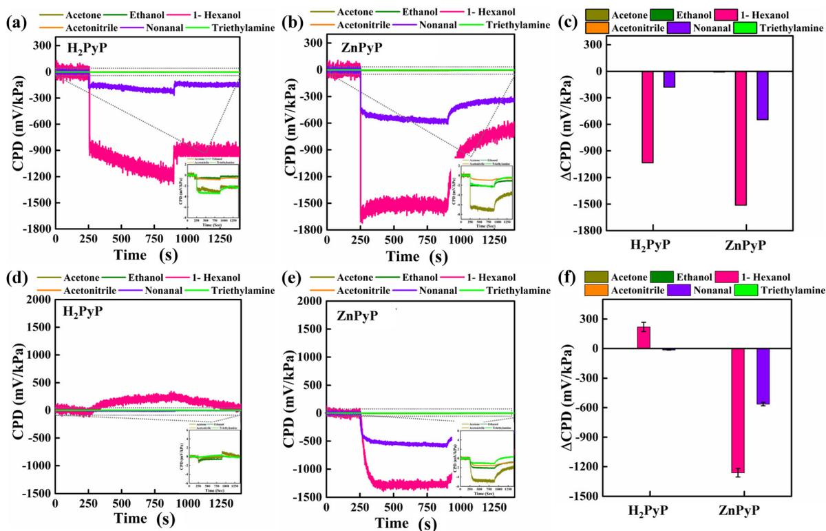
Fig. 5 Single-point CPD plots under UV light illumination for H<sub>2</sub>PyP (a) and ZnPyP (b) and under visible light illumination for H<sub>2</sub>PyP (d) and ZnPyP (e) with different VOCs. Change in the ΔCPD plots of H<sub>2</sub>PyP and ZnPyP under (c) UV and (f) visible light illumination upon VOCs exposure.
