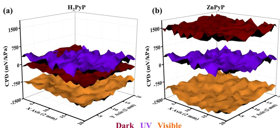
Fig. 6 3D raster scan images of 1-hexanol for (a) H<sub>2</sub>PyP and (b) ZnPyP under dark, UV, and visible light illumination.
