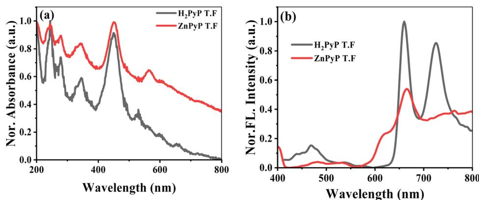
Fig. 1 Absorption spectra of H<sub>2</sub>PyP and ZnPyP coated on a quartz substrate (a). (b) Emission spectra of H<sub>2</sub>PyP and ZnPyP thin films upon excitation at  $\lambda_{\text{ex}}$  = 330 nm.
