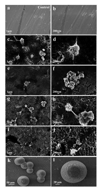
Fig. 7 SEM images of the control and the treated samples taken using the in-lens detector after immersion in SBF solution for 1 week; (a) and (b) control; the treated surfaces show the nucleation of apatite (c) and (d) NNa5; (e) and (f) NaN5; (g) and (h) NNa10; (i) and (j) NaN10; (k) and (l) low magnification, large apatite formation on the surface of NaN5 and NNa10.
