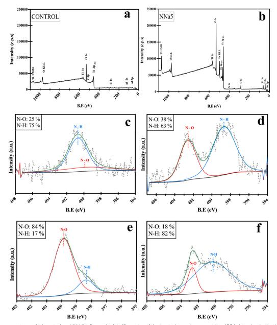
Fig. 5 XPS survey spectrum of (a) control and (b) NNa5 sample; (c)–(f) spectra of the treated samples around the 400 keV region indicating the presence of nitrogen in NO and NH bonds: (c) NNa5, (d) NaN5, (e) NNa10 and (f) NaN10.
