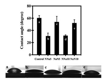
Fig. 3 Plot of water contact angles of the untreated and treated samples; (a) untreated (control), (b) NNa5, (c) NaN5, (d) NNa10 and (e) NaN10
