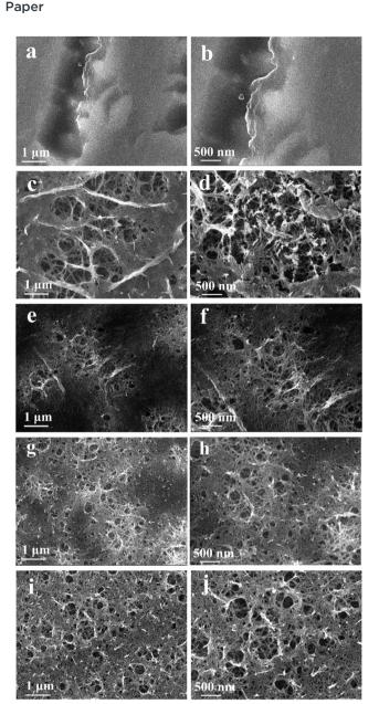
SEM images of the samples taken using the in-lens detector after dual alkaline etching for 24 h; (a) and (b) untreated sample; (c) and (d) NNa5; (e) and (f) NaN5; (g) and (h) NNa10 and (i) and (j) NaN10.
