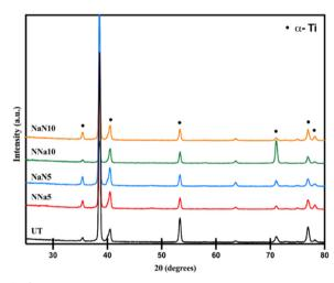
Fig. 4 GIXRD pattern of the dual alkali treated groups and the untreated samples at room temperature.
