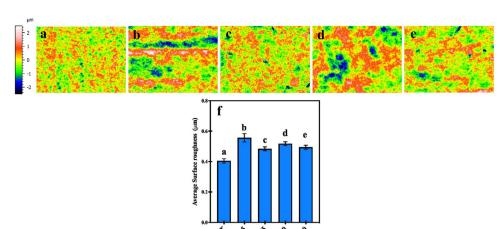
Fig. 2 (a)-(e) Results of optical profilometry measurements of the samples - difference in surface topography is indicated by the color scale; (a) untreated, (b) NNa5, (c) NaN5, (d) NNa10 and (e) NaN10; (f) comparison of average surface roughness before and after the dual alkaline etching
