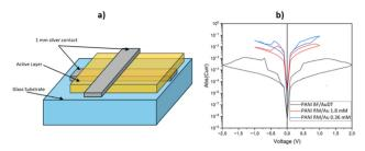
(a) Schematic layout of the fabricated devices; (b) current-voltage characteristics (plot with absolute current) of the device with PANI BF/ AuDT, PANI RM/Au 1.8 mM and PANI RM/Au 0.36 mM
