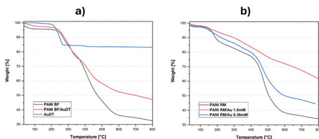
Fig. 1 TGA curves of (a) AuDT, PANI BF and PANI BF/AuDT as well as (b) PANI RM/Au.
