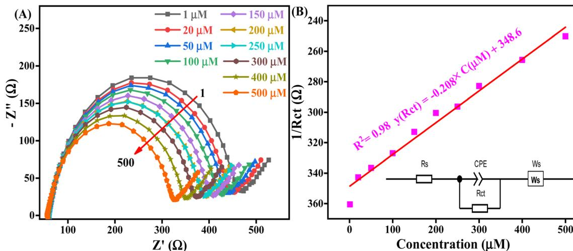
Fig. 7 (A) EIS spectra of the Nyquist plot on the nanofabricated La/CF/rGO/ITO bioelectrode from 1 to 500  $\mu\text{M}$ , expressed in Ohm, and (B) biosensing linear calibration curve of AD, expressed in between the  $1/R_{ct}$  versus different concentrations of AD at OEP, and the inset shows the equivalent circuit.
