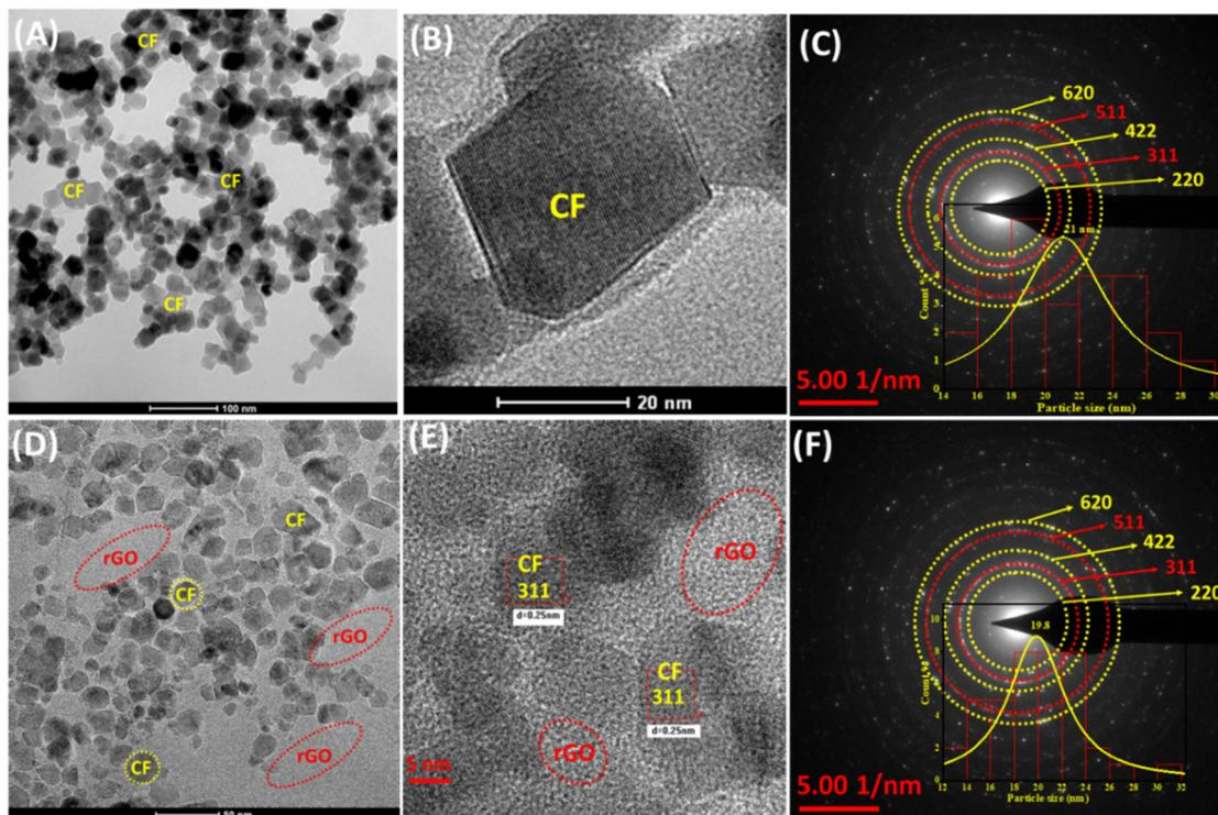
**Fig. 2** (A) and (B) HR-TEM microimages of CF with rectangular morphology, (C) SAED pattern of CF with equivalent planes confirmed by JCPDS  $d$ -spacing value, and the inset histogram shows the average particle size, (D) and (E) HR-TEM microimages of mesoporous CF/rGO nh indicating lattice fringes equivalent to high-intensity planes, and (F) the SAED pattern of mesoporous CF/rGO nh with equivalent planes confirmed by JCPDS  $d$ -spacing and average particle size histogram.
