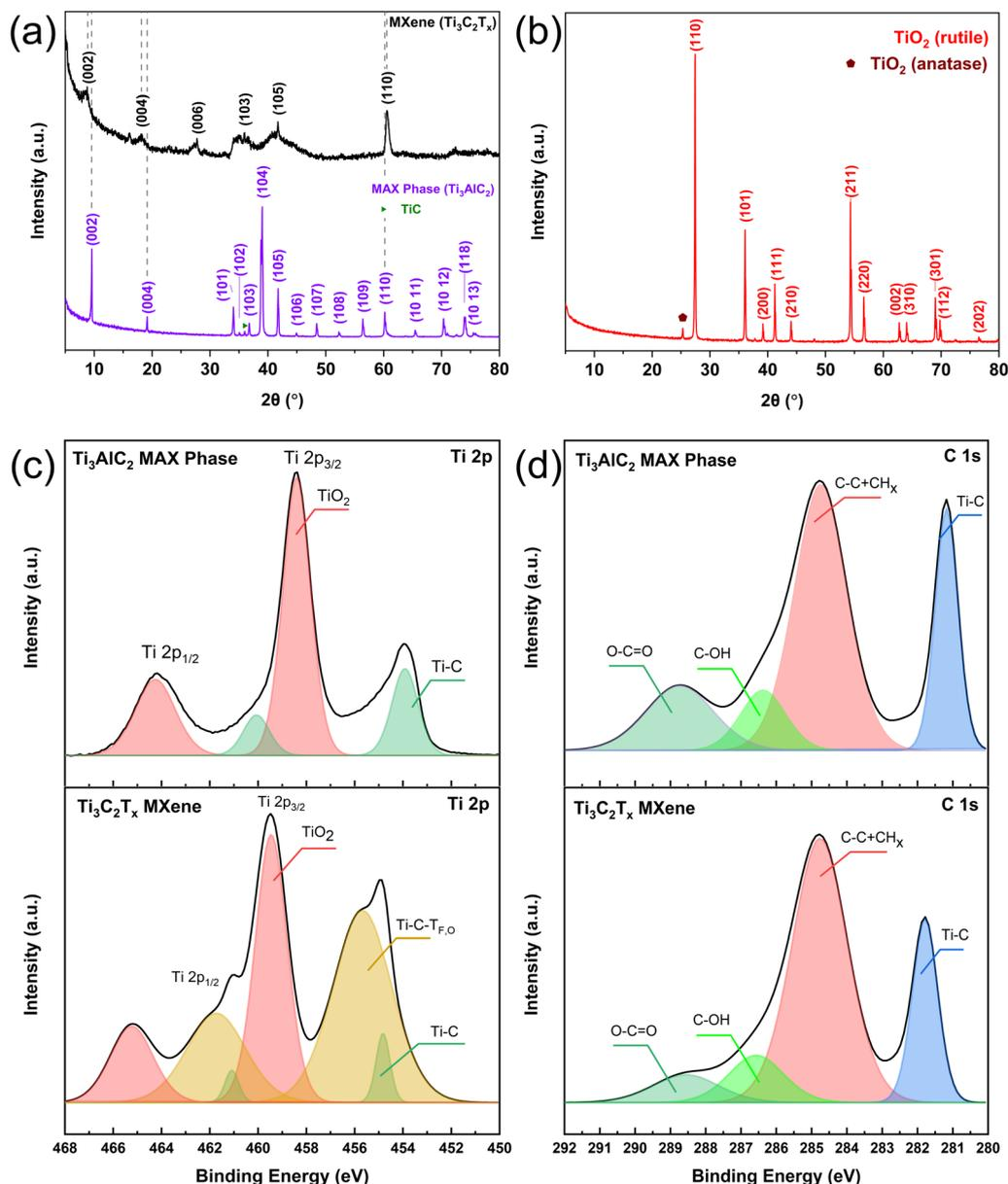
Fig. 2 XRD patterns of the (a) MAX phase and MXene, (b)  $\text{TiO}_2$ ; high-resolution XPS spectra of (c) Ti 2p and (d) C 1s in the  $\text{Ti}_3\text{AlC}_2$  MAX phase and  $\text{Ti}_3\text{C}_2\text{T}_x$  MXene samples.
