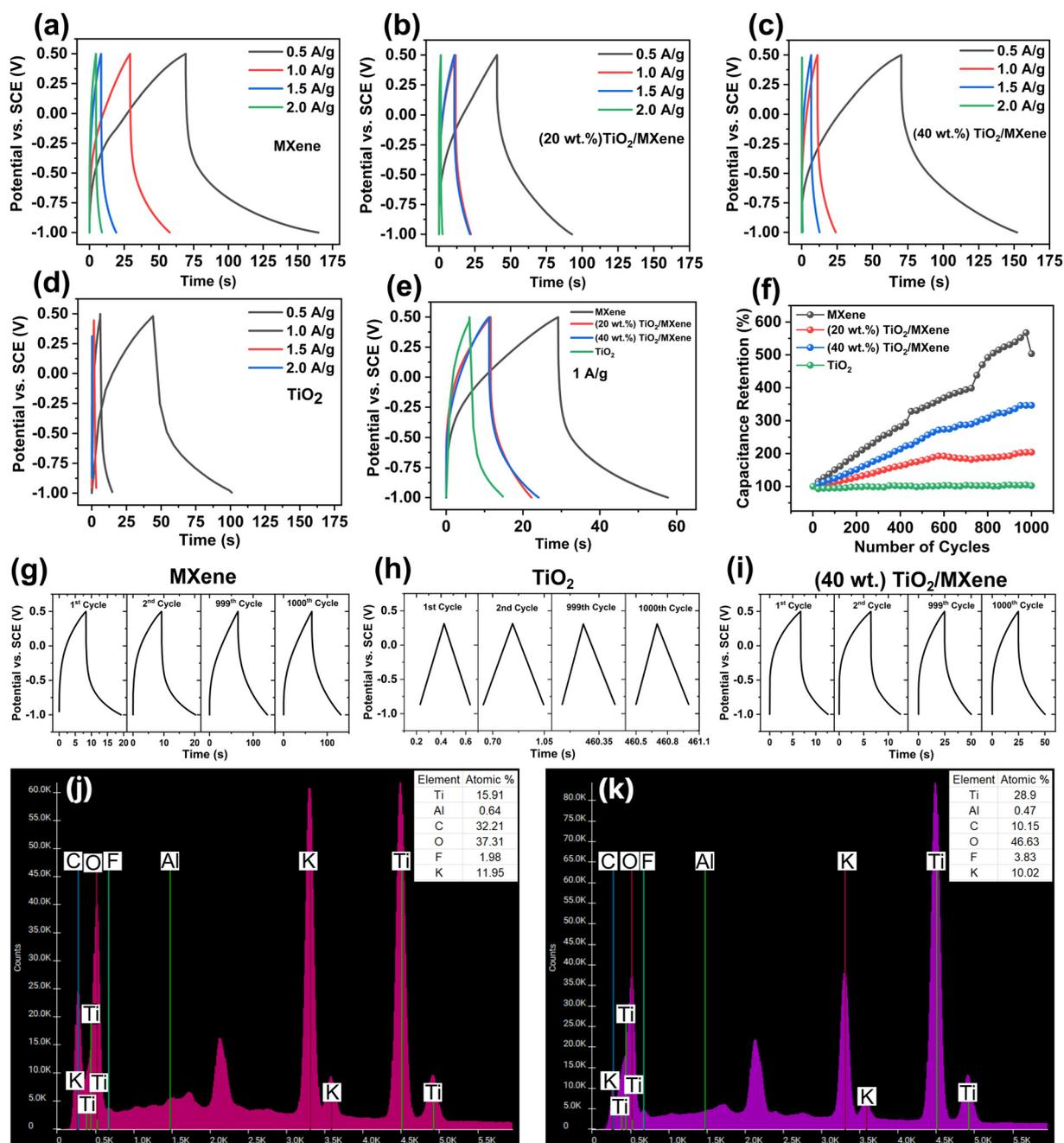
Fig. 6 The GCD data for fabricated electrodes. (a)–(d) at multiple current densities; (e) at a  $1\ A\ g^{-1}$  constant current density; (f) capacitance retention graph at a  $1.5\ A\ g^{-1}$  current density; (g)–(i) potential profiles during cycling for MXene,  $TiO_2$ , and (40 wt.)  $TiO_2$ /MXene; EDS spectrum data for (j) MXene and (k) (20 wt%)  $TiO_2$ /MXene electrodes after 1000 charging–discharging cycles.
