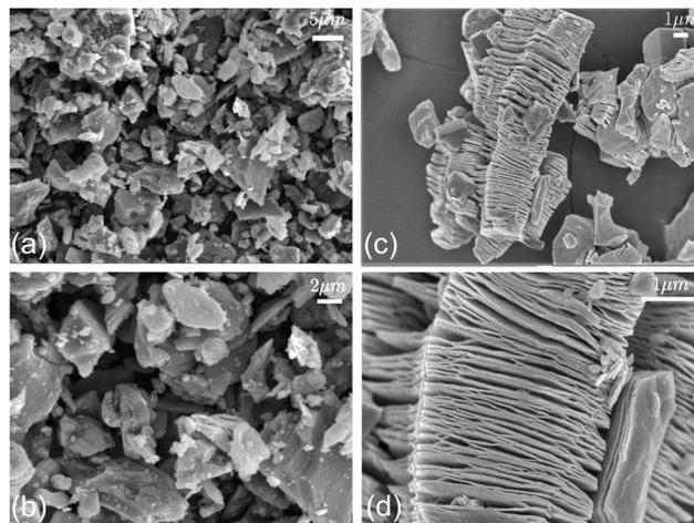
**Fig. 3** SEM images of the (a) and (b) MAX phase (Ti<sub>3</sub>AlC<sub>2</sub>) and (c) and (d) synthesized MXene (Ti<sub>3</sub>C<sub>2</sub>T<sub>x</sub>) at (a), (c) 5000×, (b) 10 000×, and (d) 20 000× magnifications.
