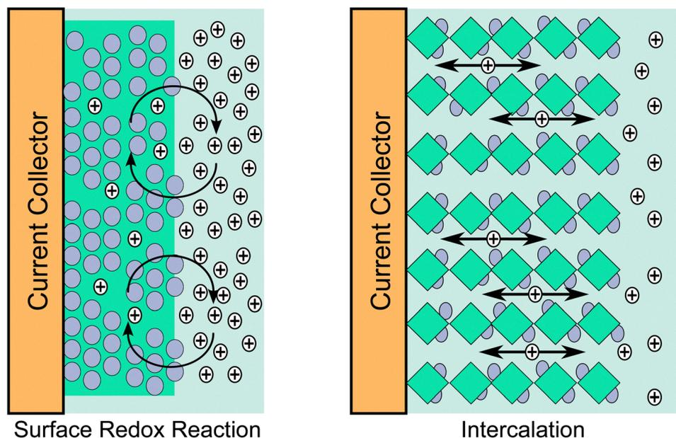
**Fig. 7** A schematic diagram illustrating the surface redox reaction and intercalation mechanisms for energy storage in pseudocapacitors.
