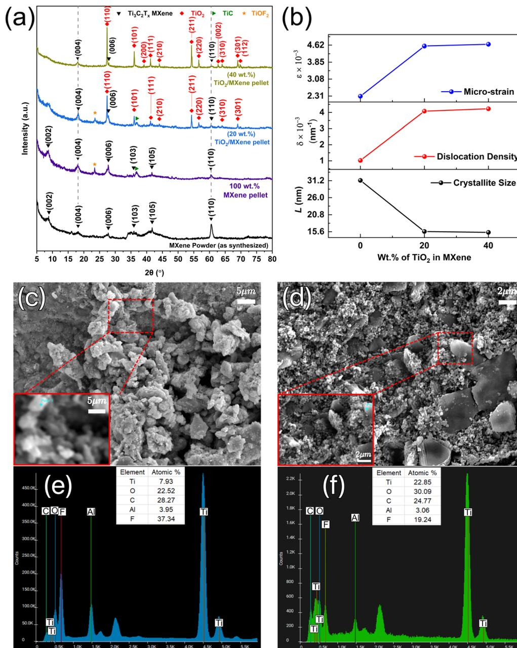
Fig. 4 (a) XRD patterns for as-synthesized MXene powder and cold-sintered nanocomposite pellets, (b) the variation of the crystallite size ( $L$ ), dislocation density ( $\delta$ ), and micro-strain ( $\epsilon$ ) as a function of the weight percentage of TiO<sub>2</sub> in the MXene cold-sintered at 150 °C temperature and 150 MPa pressure, and the SEM-EDS images of the (c) and (e) (20 wt%) TiO<sub>2</sub>/MXene and (d) and (f) (40 wt%) TiO<sub>2</sub>/MXene nanocomposites.
