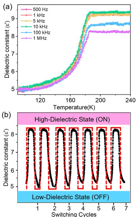
Fig. 4 (a) Switchable  $T$ - $\epsilon'$  curves of **1** measured in the range from 500 Hz to 1 MHz (in the heating process). (b)  $\epsilon'$ -switching cycles of **1** determined at 1 MHz. The dielectric property of **1** was obtained using a polycrystalline sample.
