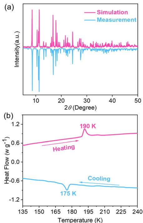
Fig. 1 (a) PXRD pattern for **1** measured at room temperature. (b) DSC curves of **1** measured in a cooling-heating cycle with a rate of 20 K min<sup>-1</sup>.
