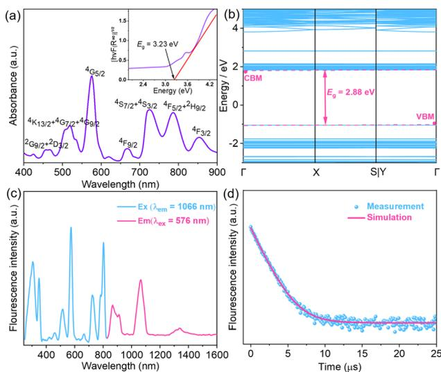
Fig. 5 NIR photoluminescent properties of **1** at room temperature. (a) Absorption spectrum. Embedded map is an absorption spectrum fitting band gap map. (b) The calculated band structure of **1**. (c) Excitation ( $\lambda_{\text{em}} = 1066$  nm) and emission ( $\lambda_{\text{ex}} = 576$  nm) spectra of **1**. (d) Fluorescence decay curve for the  ${}^4\text{F}_{3/2} \rightarrow {}^4\text{I}_{11/2}$  transition.
