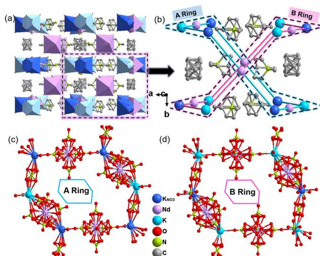
Fig. 3 (a) Packing structures of **1** at 300 K. (b) Simple diagram of the bicyclic crystal structure at 300 K. Note: the ligands of metal atoms are omitted. (c) Structure of A-ring at 300 K. (d) Structure of B-ring at 300 K. Note:  $K_{NO_3}$  stands for K atom with  $NO_3^-$  coordination. H atoms are omitted for clarity.
