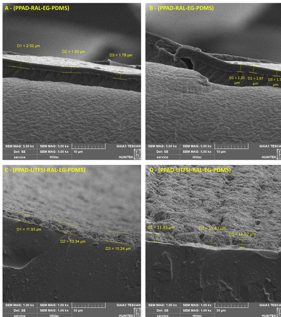
Fig. 10 Coating thickness measurements (A) and (B) PPAD-RAL-EG-PDMS, and (C) and (D) PPAD-LiTFSI-RAL-EG-PDMS.
