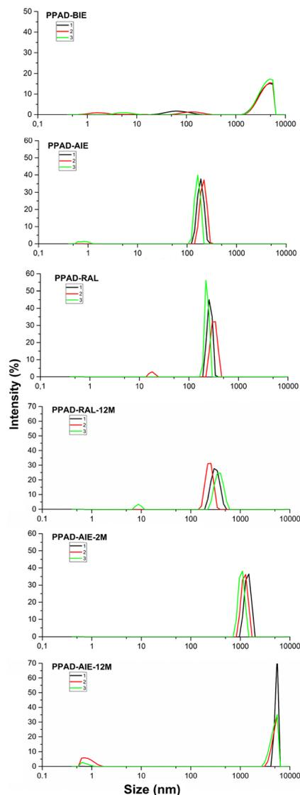
Fig. 2 PPAD-BIE, PPAD-AIE, PPAD-RAL, PPAD-RAL-12M, PPAD-AIE-2M and PPAD-AIE-12M particle size results.
