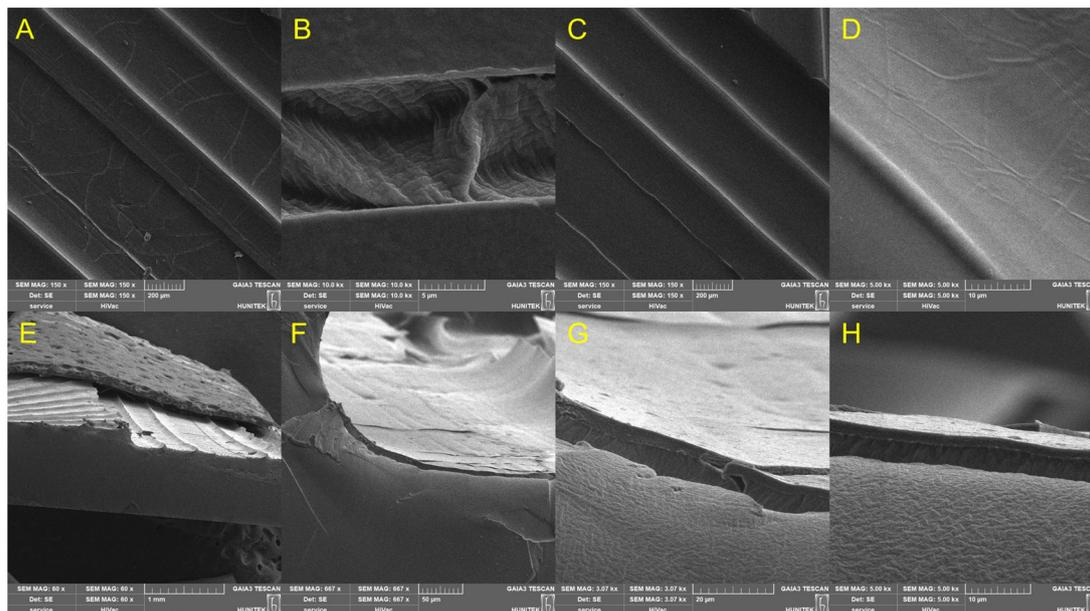
Fig. 7 SEM images of the PPAD-RAL-EG-PDMS composite. (A)–(D) The top view. (E)–(H) The cross-sectional view.
