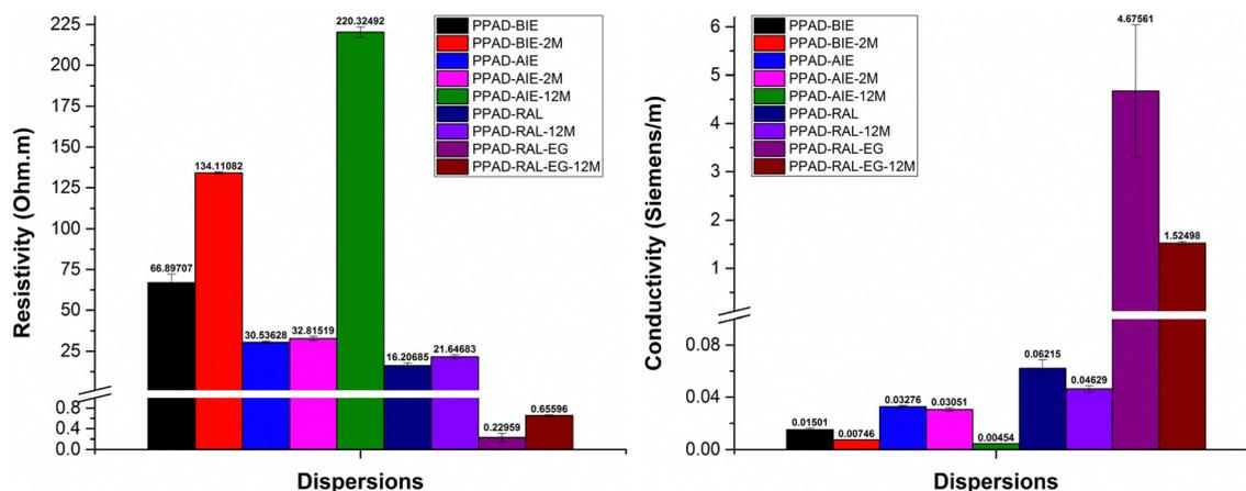
Fig. 11 PPAD group's resistivity and conductivity measurements including PPAD-BIE, PPAD-BIE-2M, PPAD-AIE, PPAD-AIE-2M, PPAD-AIE-12M, PPAD-RAL, PPAD-RAL-12M, PPAD-RAL-EG and PPAD-RAL-EG-12M.
