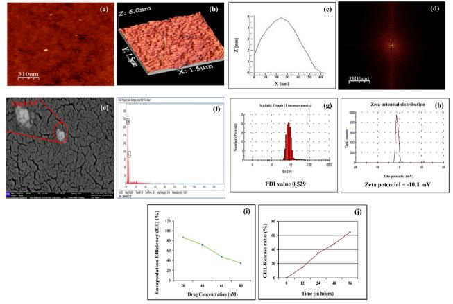
Fig. 1 (a) – (d) AFM images of NCHL: (a) 2D view of NCHL, (b) 3D view of NCHL, (c) size profile of NCHL, (d) FFT analysis, (e) FESEM image of NCHL, (f) EDX spectra of NCHL, (g) DLS spectroscopy showing the average diameter of NCHL within 0-100 nm with a PDI value of 0.529, (h) zeta potential of NCHL, (i) graphical representation of % encapsulation efficacy (%EE) of CHL in PLGA-Nps with increasing amount of drug (CHL), and (j) in vivo release kinetics of NCHL.
