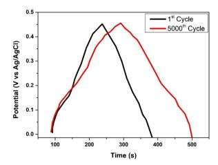
Fig. 9 Galvanostatic charge–discharge (GCD) plots of  $Sr_{0.9}X_{0.1}CoO_{3-\delta}$ (X = Ce) perovskite electrodes synthesized through the semi-green (LP) approach, comparing the electrochemical behavior between the 1st and 5000th cycles.
