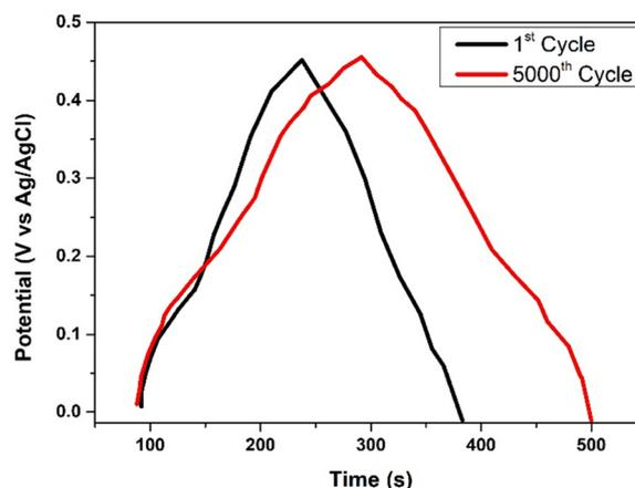
Fig. 9 Galvanostatic charge–discharge (GCD) plots of  $\text{Sr}_{0.9}\text{X}_{0.1}\text{CoO}_{3-\delta}$  (X = Ce) perovskite electrodes synthesized through the semi-green (LP) approach, comparing the electrochemical behavior between the 1st and 5000th cycles.
