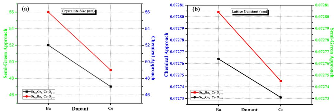
**Fig. 3** Variation of (a) crystallite size and (b) lattice constant for the (110) plane of  $\text{Sr}_{0.9}\text{X}_{0.1}\text{CoO}_{3-\delta}$  ( $X = \text{Ba}, \text{Ce}$ ) synthesized through semi-green (LP) and chemical (CA) approaches.
