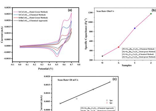
Fig. 8 (a) Cyclic voltammetry curves of  $Sr_{0.9}X_{0.1}CoO_{3-\delta}$  (X = Ba, Ce) within the potential window range of -0.1 to 0.7 V at a scan rate of 20 mV s<sup>-1</sup>. (b) Specific capacitance of  $Sr_{0.9}X_{0.1}CoO_{3-\delta}$  (X = Ba, Ce). (c) Anodic and cathodic peak currents obtained from the CV curves of  $Sr_{0.9}X_{0.1}CoO_{3-\delta}$  (X = Ba, Ce). Ce) synthesized through the semi-green (LP) and chemical (CA) approaches.
