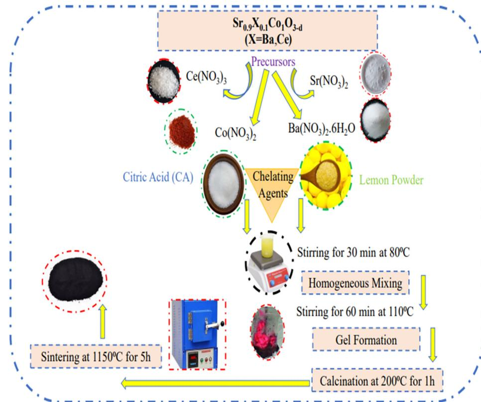
Fig. 1 Schematic of  $\text{Sr}_{0.9}\text{X}_{0.1}\text{CoO}_{3-\delta}$  ( $\text{X} = \text{Ba}, \text{Ce}$ ) perovskite anode materials synthesized through semi-green (LP) and chemical (CA) approaches.
