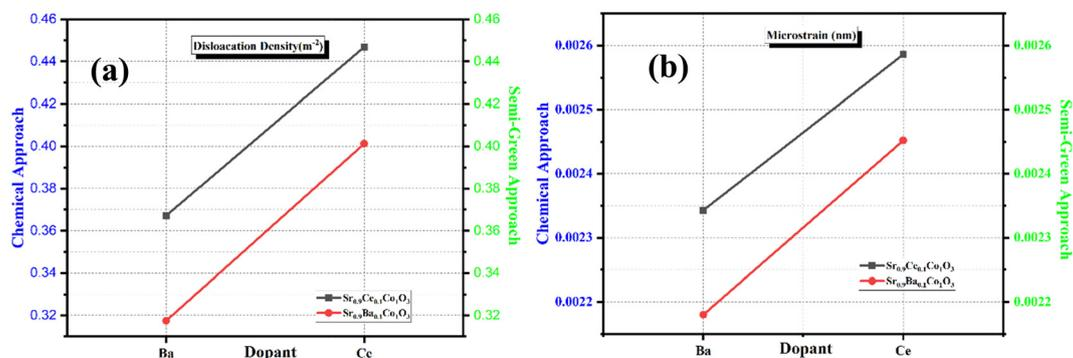
**Fig. 4** Variation of (a) dislocation density and (b) microstrain for the (110) plane of  $\text{Sr}_{0.9}\text{X}_{0.1}\text{CoO}_{3-\delta}$  ( $X = \text{Ba}, \text{Ce}$ ) synthesized through the semi-green (LP) and chemical (CA) approaches.
