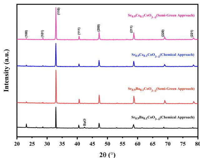
Fig. 2 XRD spectra of  $\text{Sr}_{0.9}\text{X}_{0.1}\text{CoO}_{3-\delta}$  ( $\text{X} = \text{Ba}, \text{Ce}$ ) synthesized through semi-green and chemical approaches, showing the cubic perovskite structure for all samples with no extra phases. However, a small BaO phase appeared for  $\text{Sr}_{0.9}\text{Ba}_{0.1}\text{CoO}_{3-\delta}$  synthesized through the chemical approach.
