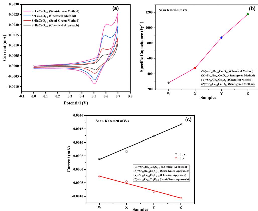
Fig. 8 (a) Cyclic voltammograms of  $\text{Sr}_{0.9}\text{X}_{0.1}\text{CoO}_{3-\delta}$  (X = Ba, Ce) within the potential window range of -0.1 to 0.7 V at a scan rate of 20 mV s<sup>-1</sup>. (b) Specific capacitance of  $\text{Sr}_{0.9}\text{X}_{0.1}\text{CoO}_{3-\delta}$  (X = Ba, Ce). (c) Anodic and cathodic peak currents obtained from the CV curves of  $\text{Sr}_{0.9}\text{X}_{0.1}\text{CoO}_{3-\delta}$  (X = Ba, Ce) synthesized through the semi-green (LP) and chemical (CA) approaches.
