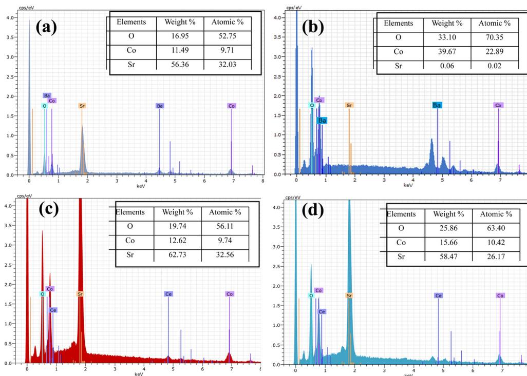
Fig. 6 EDX spectra of  $\text{Sr}_{0.9}\text{X}_{0.1}\text{CoO}_{3-\delta}$  (a) doped with (X = Ba) using citric acid as a chelating agent, (b) doped with (X = Ba) using lemon powder as a chelating agent, (c) doped with (X = Ce) using citric acid as a chelating agent, and (d) doped with (X = Ce) using lemon powder as a chelating agent.
