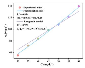
Fig. 7 Adsorption isotherm  $q_e - C_{p-NP}$  curves of the adsorption of p-NP by Eu-MOF fitted by the Freundlich and Langmuir models.
