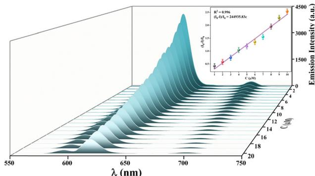
Fig. 4 Emission spectra of Eu-MOF after sequential dropping of 10  $\mu$ L of 0.1 mM *p*-NP, with the plot of  $I_0/I$  vs.  $C_{p-NP}$  in the inset.
