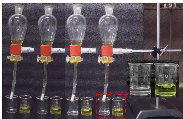
**Fig. 10** Pictures of  $p$ -NP filtrated through a Pd@Eu-MOF@SA stopper in a separatory funnel.
