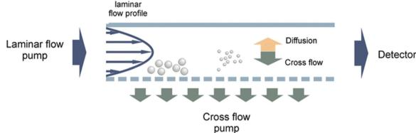
Fig. 13 Asymmetric field-flow fractionation (AF4): prior to separation, samples are concentrated on the membrane. Particles diffuse off the membrane based on their size, aggregating in regions where the forces of diffusion and cross flow are balanced. Concurrently, laminar flow directs the particles toward the detector located at the end of the flow channel. This figure is reproduced from ref. 73 with permission from Sensors, copyright (2023).
