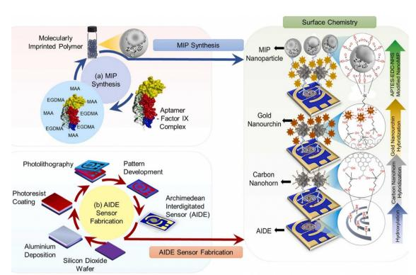
Fig. 11 Schematic overview of the entire investigation: this includes the synthesis of molecularly imprinted polymers (MIPs) (a) and the fabrication of the AIDE sensor through photolithography (b). This figure is reproduced from ref. 69 with permission from Elsevier, copyright (2022).
