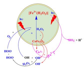
Fig. 30 Mechanism of decomposition of H<sub>2</sub>O<sub>2</sub> solution in the presence of the CFO nanoparticles as catalyst.
