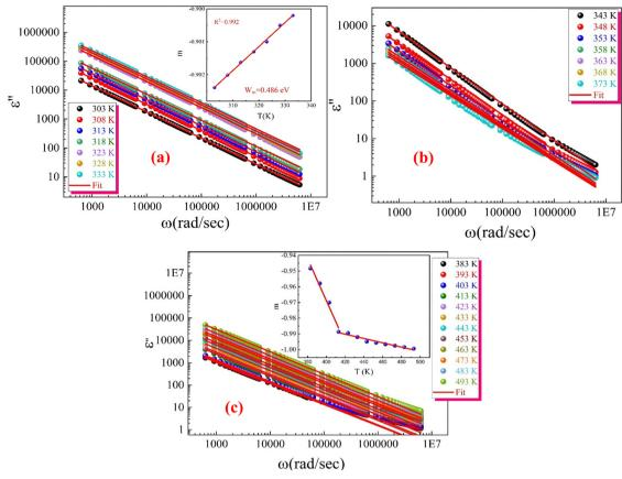
Fig. 24 Giuntini model fit for the imaginary part of the permittivity  $\varepsilon''$  with the angular frequencies (a) at the first temperature region (303–333 K), (b) at the second temperature region (343–373 K), and (c) at the third temperature region (383–493 K) for the synthesized CFO ferrite nanoparticles. The inset shows the temperature dependence of the exponent factor m.
