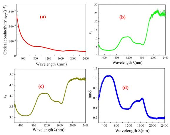
Fig. 11 (a) Optical conductivity as a function of wavelength ( $\lambda$ ) (b) real part of the optical dielectric permittivity  $\varepsilon_1$  as a function of wavelength ( $\lambda$ ) (c) imaginary part of the optical dielectric permittivity  $\varepsilon_2$  as a function of wavelength ( $\lambda$ ) (d) optical loss factor tan ( $\delta$ ) as a function of wavelength ( $\lambda$ ) for the green-syenthesized CFO nanoparticles
