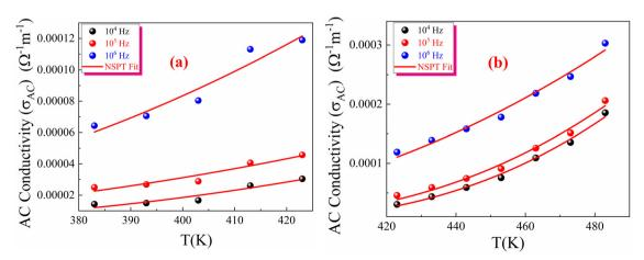
Fig. 19 Temperature dependence of the NSPT fitting model for the AC conductivity of green-synthesized CFO nanoparticles in the temperature range of (a) 383 to 423 K (b) 423 to 493 K
