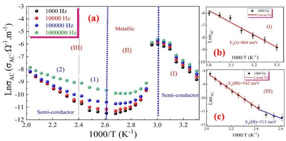
Fig. 21 (a) Variation of  $\ln \sigma_{ac}$  versus 1000/T for the green synthesized CFO nanoparticles as a function of applied field frequencies, (b) and (c) show magnified views of the linear fits in regions (I) and (III) at low (303-333 K) and high (383-493 K) temperatures, respectively.
