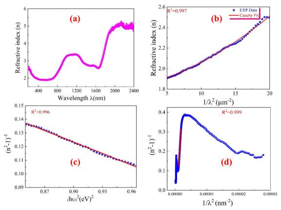
Fig. 10 (a) Variation of refractive index (n) as a function of the incident photon wavelength ( $\lambda$ ). (b) Variation of ( $n(\lambda)$ ) with Cauchy fit. (c) The Plot of  $1/(n^2-1)$  versus ( $h\nu$ )<sup>2</sup> (d) plot of  $1/(n^2-1)$  versus  $1/\lambda^2$  for the green-synthesized CFO nanoparticles.
