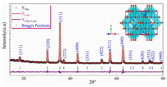
Fig. 1 Rietveld refinements of the powder diffraction pattern of the CFO nanoparticles. The inset shows the polyhedron configuration of the facecentred cubic spinel structure of CFO.21
