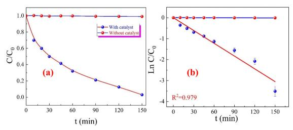
Fig. 29 (a) Time-dependent profile of  $H_2O_2$  degradation with and without catalyst (b)  $ln(C_0/C_t)$  versus time.
