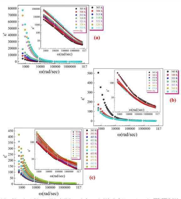
Fig. 22 Variation of the real part of the permittivity  $\varepsilon'$  with the angular frequencies (a) for the first temperature region (303–333 K), (b) for the second temperature region (343–373 K), and (c) for the third temperature region (383–493 K) for the synthesized CFO ferrite nanoparticles. The inset shows the H–N model fitting.
