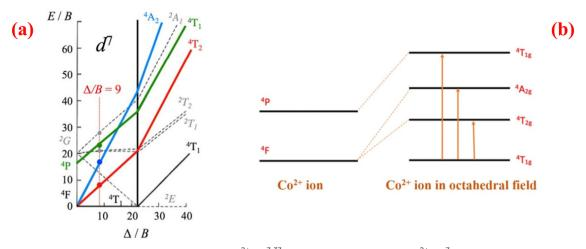
Fig. 3 (a) Simplified Tanabe-Sugano diagram for octahedral  $Co^{2+}$  ( $3d^7$ ) $^{37}$  (b) The energy levels of the  $Co^{2+}$  ( $3d^7$ ) ion in an octahedral field with three spin allowed electronic transitions from d to d in CoO<sub>6</sub>.
