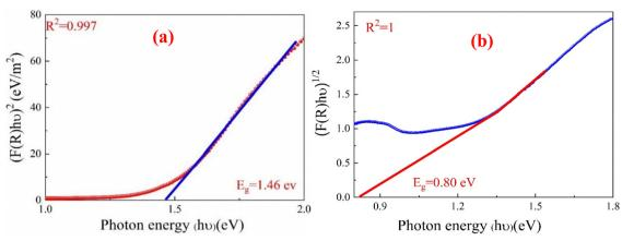
Fig. 5 (a)  $(F(R)h\nu)^2$  spectra versus the photon energy  $(h\nu)$  for direct band gap energy.<sup>21</sup> (b)  $(F(R)h\nu)^{1/2}$  spectra versus the photon energy  $(h\nu)$  for indirect band gap energy for the eco-friendly CFO nanoparticles.
