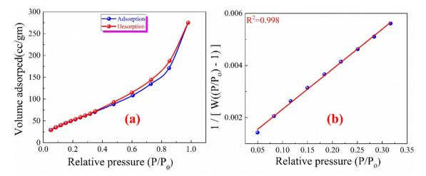
Fig. 27 (a) N<sub>2</sub> adsorption-desorption isotherm (b) Brunauer-Emmett-Teller plot of the CFO nanoparticles.<sup>21</sup>
