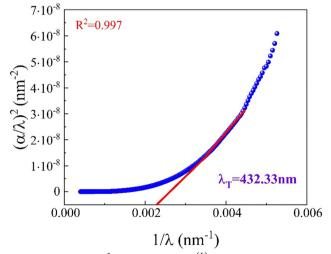
Fig. 7 Variation of  $\left(\frac{\alpha}{\lambda}\right)^2$  as a function of  $\left(\frac{1}{\lambda}\right)$  to estimate the threshold wavelength  $(\lambda_T)$ .
