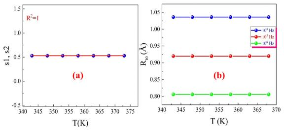
Fig. 16 (a) Temperature variation of the exponents "s". (b) Thermal variation of the tunnelling distance  $R_{\omega}$  as a function of the frequency of the applied electric field for the eco-friendly synthesized CFO nanoparticles within the temperature range of 343–373 K.
