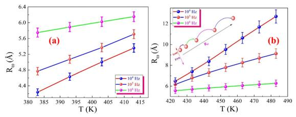
Fig. 20 Temperature-dependent variation of the tunnelling distance  $R_{\omega}$  at different frequencies for the eco-friendly synthesized CFO nanoparticles within the temperature range of (a) 383–413 K and (b) 423–493 K.
