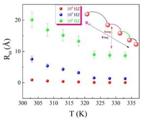
Fig. 15 Temperature-dependent variation of the hopping distance  $R_{\infty}$  at different frequencies for the eco-friendly synthesized CFO nanoparticles within the 303-333 K temperature range.
