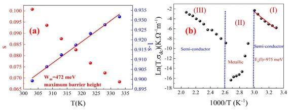
Fig. 13 (a) Temperature variation of the exponents "s" and "1 - s" within the temperature range of 303–333 K (b) Plot of  $\ln(\sigma_{dc}T)$  as a function of (1000/T) within the temperature range of 303–490 K for the eco-friendly synthesized CFO nanoparticles.
