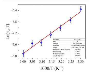
Fig. 26 Arrhenius plot of  $ln(\tau \times T)$  versus (1000/T) for the green-synthesized CFO nanoparticles.
