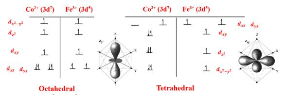
Fig. 4 Crystal field splitting of Fe<sup>3+</sup> and Co<sup>2+</sup> cation 3d orbitals for tetrahedral and octahedral symmetries. Net spins have been illustrated for every conceivable cation-charge state
