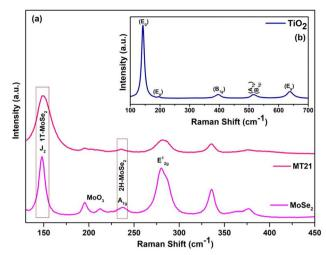
Fig. 1 Raman spectra of (a) MoSe<sub>2</sub> and the MoSe<sub>2</sub>/TiO<sub>2</sub> (2:1) composite and (b) TiO<sub>2</sub>
