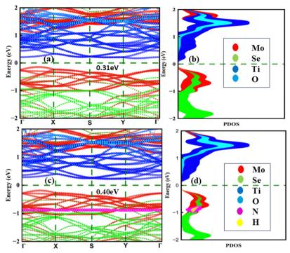
Fig. 6 (a) and (c) Electronic band structure and (b) and (d) projected density of state of the MoSe<sub>2</sub>/TiO<sub>2</sub> heterostructure and after NH<sub>3</sub> adsorbed on the heterostructure, respectively, using the GGA + PBE method.
