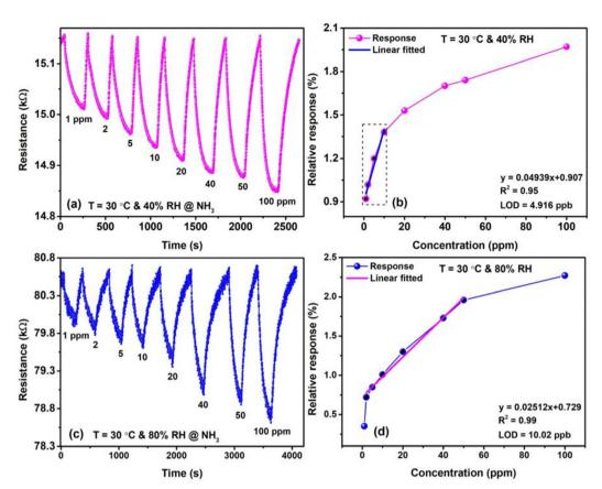
Fig. 3 (a) and (c) Response transient curves for the  $MoSe_2/TiO_2$  (2:1) sensor exposed to various concentrations of  $NH_3$  ranging from 1 to 100 ppm at 30 °C and relative humidity (RH) levels of 40% and 80%. (b) and (d) Relative response *versus*  $NH_3$  concentration curves at 40% and 80% RH.
