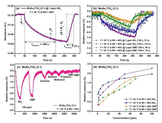
Fig. 4 (a) A representative response-recovery transient for the  $MoSe_2/TiO_2$  (2:1) sensor with 1 ppm ammonia at 30 °C and 40% RH. (b) Sensing response of the  $MoSe_2/TiO_2$  (2:1) composite sensor for different humidities and different analytes. (c) Selectivity tests for the  $MoSe_2/TiO_2$  (2:1) composite sensor to various gases at room temperature. (d) Relative response vs concentration in different humidities and different analytes (NH<sub>3</sub> and DMF).
