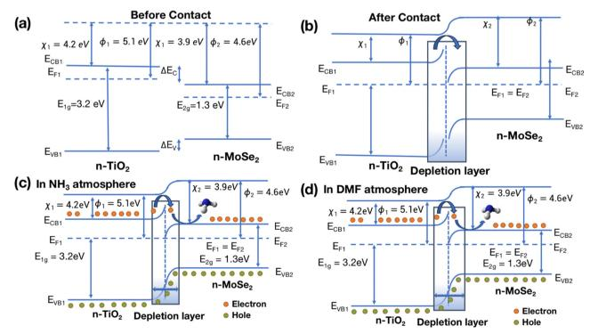
Fig. 8 (a) and (b) Simulated energy band diagram before and after contact and schematic showing the NH<sub>3</sub> sensing mechanism (c) and (d) in the NH<sub>3</sub> and DMF gas atmosphere, for the MoSe<sub>2</sub>/TiO<sub>2</sub> heterojunction.
