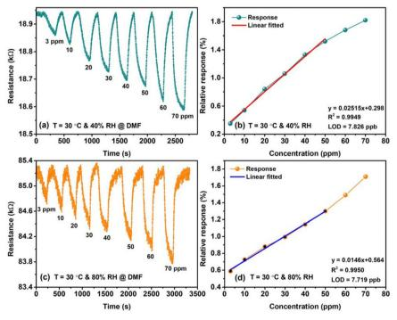
Fig. 5 (a), (c) Response transient curves for the MoSe $_2$ /TiO $_2$  (2:1) sensor when exposed to varying concentrations of DMF from 3 to 70 ppm at 30  $^{\circ}$ C and relative humidity (RH) levels of 40% and 80%. (b) and (d) Relative response *versus* DMF concentration curves at 40% and 80% RH.
