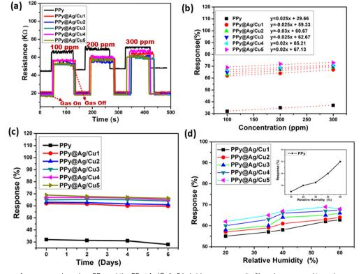
Fig. 12 (a) Resistance of gas sensors based on PPy and the PPy@Ag/Cu1-5 hybrid nanocomposite film when exposed to various concentrations of NH $_3$  gas at room temperature, (b) sensitivity of PPy and its hybrid nanocomposite film, (c) stability of the gas sensor based on PPy and its nanocomposite film toward 100 ppm ammonia and (d) effect of humidity on the prepared sensor when exposed to 100 ppm ammonia.
