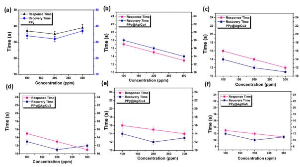
Fig. 13 Response-recovery curves of gas sensors based on the (a) PPy and (b) and (f) PPy@Aq/Cu hybrid nanocomposite film when exposed to various concentrations of NH<sub>3</sub> gas at room temperature.
