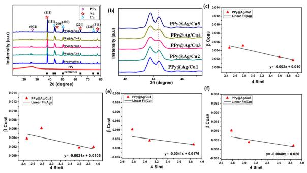
Fig. 5 (a) The XRD spectra of the PPy and PPy@Ag/Cu1-5 hybrid nanocomposite; (b) magnified view of the XRD pattern for the Ag peak shift on the (200) plane of the PPy@Ag/Cu hybrid nanocomposite; (c-f) Williamson-Hall plot of the nano-crystalline silver and copper sample
