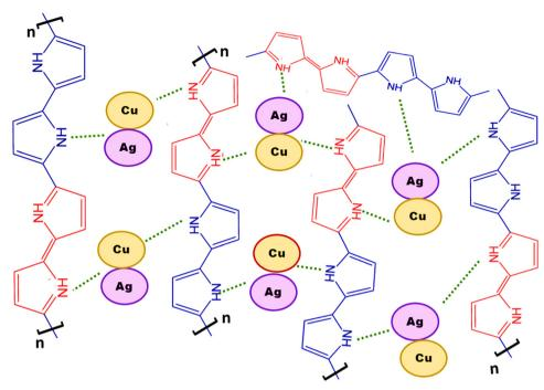
Fig. 3 Stabilization mechanism of the PPy@Ag/Cu hybrid nanocomposite.
