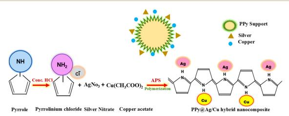
Fig. 2 Synthesis of the PPy@Ag/Cu hybrid nanocomposite.
