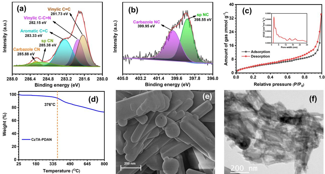
Fig. 2 (a) High-resolution C 1s XPS spectrum and (b) high-resolution N 1s XPS spectrum of the CzTA-PDAN COP. (c) N<sub>2</sub> isotherm of the CzTA-PDAN at 77 K. (d) TGA curve of the CzTA-PDAN COP. (e) FE-SEM image and (f) TEM image of the CzTA-PDAN COP at 200 nm resolution.
