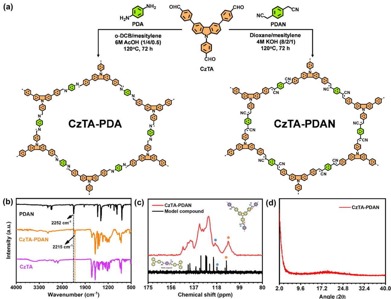
Fig. 1 (a) Synthesis of the CzTA-PDAN COP under solvothermal conditions. (b) FT-IR spectra of the CzTA-PDAN COP. (c) Solid-state  $^{13}\text{C}$  CP-MAS NMR spectra of the CzTA-PDAN COP. (d) PXRD pattern of the CzTA-PDAN COP.
