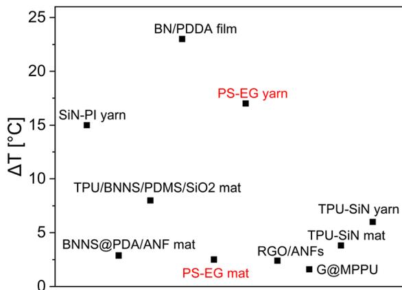
Fig. 5 The comparison of the thermal performance of our work with recently published literature,<sup>4,22,97–101</sup> where  $\Delta T$  means thermal improvement of composite fiber compared to either pristine polymer, cotton or other reference material.
