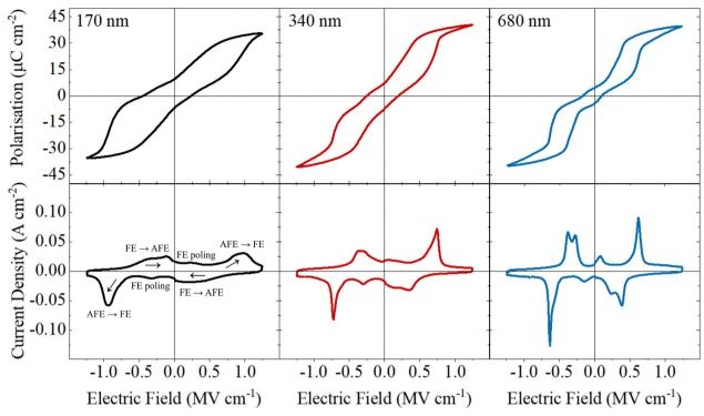
Fig. 4 P(E) and j(E) loops of the PbZrO $_3$  films with different thicknesses. The measurements were performed at 100 Hz.
