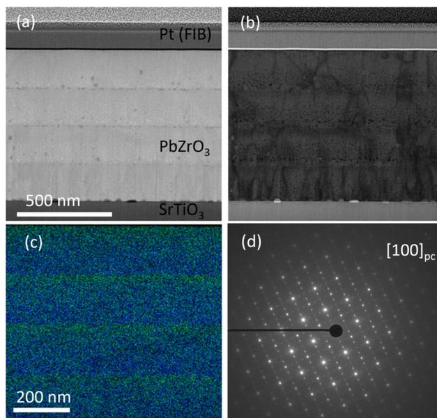
**Fig. 3** STEM images of a 680 nm-thick film. High-angle annular dark-field (HAADF) (a) and bright-field (BF) (b) STEM micrographs of 680 nm-thick film. (c) Composite EDXS image of PbZrO<sub>3</sub> film using Zr K (green) and Pb M lines (blue). (d) Selected area diffraction pattern (SAED) of the PbZrO<sub>3</sub> film in [100]<sub>pc</sub> zone axis showing  $\frac{1}{4}$  superlattice spots in  $\langle 110 \rangle$  directions.
