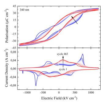
Fig. 5 P(E) and j(E) loops of a 340 nm-thick film after different number of cycles.
