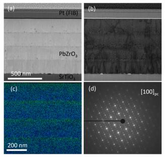
Fig. 3 STEM images of a 680 nm-thick film. High-angle annular dark-field (HAADF) (a) and bright-field (BF) (b) STEM micrographs of 680 nm-thick film. (c) Composite EDXS image of PbZrO $_3$  film using Zr K (green) and Pb M lines (blue). (d) Selected area diffraction pattern (SAED) of the PbZrO $_3$  film in [100] $_{\rm pc}$  zone axis showing  $\frac{1}{4}$  superlattice spots in  $\langle 110 \rangle$  directions.
