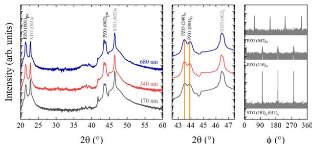
Fig. 1 X-ray diffraction (XRD) analysis of the films. (a)  $\theta$ – $2\theta$  patterns of the  $\text{PbZrO}_3$  films with different thicknesses. (b) Detailed view around the  $(240)_{\text{O}}$  and  $(004)_{\text{O}}$   $\text{PbZrO}_3$  peaks (vertical lines denote their position according to PDF file No. 01-089-1296. All non-marked peaks correspond to the substrate. (c)  $\phi$ -scans of the 170 nm-thick film.
