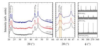
Fig. 1 X-ray diffraction (XRD) analysis of the films. (a)  $\theta$ –2 $\theta$  patterns of the PbZrO<sub>3</sub> films with different thicknesses. (b) Detailed view around the (240)<sub>O</sub> and (004)<sub>O</sub> PbZrO<sub>3</sub> peaks (vertical lines denote their position according to PDF file No. 01-089-1296. All non-marked peaks correspond to the substrate. (c)  $\phi$ -scans of the 170 nm-thick film.
