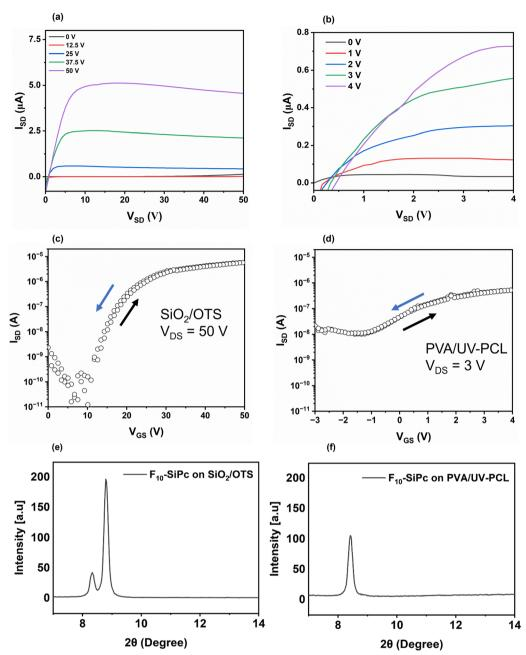
Fig. 4 Output curves of (a) SiO<sub>2</sub>/OTS and (b) PVA/UV-PCL, and transfer curves of (c) OTFT on OTS treated SiO<sub>2</sub> and (d) on PVA/UV-PCL. The transfer characteristics curve versus  $V_{GS}$  were obtained for  $V_{SD} = 50$  V and  $V_{SD} = 3$  V, respectively. 1D XRD pattern for  $F_{10}$ -SiPc on (e) OTS treated SiO<sub>2</sub> and (f) on the PVA-UV-PCL dielectric.
