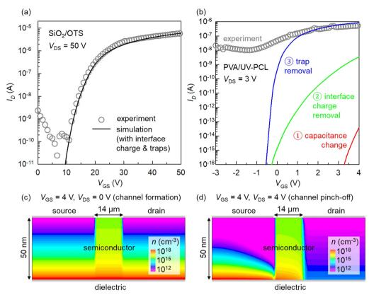
Fig. 5 Comparison between experimentally measured and numerically simulated transfer curves of the OTFT based on (a) SiO<sub>2</sub>/OTS and (b) PVA/UV-PCL dielectrics. Electron density (n) distribution on a log scale showing (c) channel formation and (d) pinch-off achieved by a low voltage in the OTFT based on the PVA/UV-PCL dielectric
