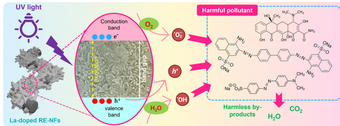
Fig. 7 Proposed photocatalytic mechanism for La-doped RE-NFs under UV light irradiation. The La-doped RE-NFs absorb UV light.
