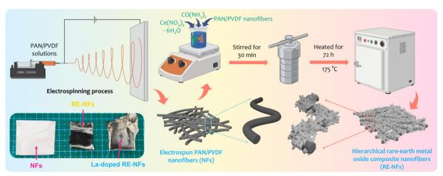
Fig. 1 Fabrication process steps for three-dimensional (3D) hierarchical rare-earth metal oxide composite nanofiber membranes. Electrospinning and hydrothermal synthesis methods are used to create polyacrylonitrile/polyvinylidene fluoride (PAN/PVDF) nanofibers and grow rare-earth metal oxide nanorods on them, respectively
