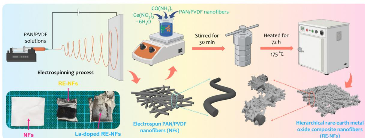
**Fig. 1** Fabrication process steps for three-dimensional (3D) hierarchical rare-earth metal oxide composite nanofiber membranes. Electrospinning and hydrothermal synthesis methods are used to create polyacrylonitrile/polyvinylidene fluoride (PAN/PVDF) nanofibers and grow rare-earth metal oxide nanorods on them, respectively.
