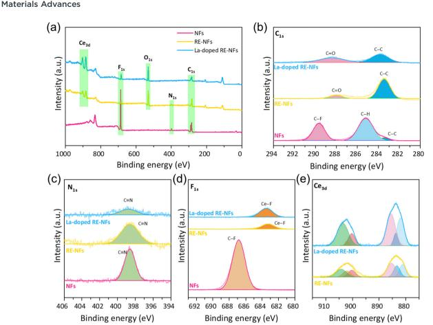
Fig. 4 XPS spectra of NFs, RE-NFs, and La-doped RE-NFs. (a) Survey spectrum displaying the elemental composition with highlighted peaks for Ce 3d, F 1s, O 1s, C 1s, and N 1s, confirming successful integration of rare-earth elements. The high-resolution spectra for (b) C 1s, (c) N 1s, (d) F 1s, and (e) Ce 3d provide detailed insights into the chemical states of each element in the prepared samples.
