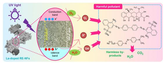
Fig. 7 Proposed photocatalytic mechanism for La-doped RE-NFs under UV light irradiation. The La-doped RE-NFs absorb UV light.
