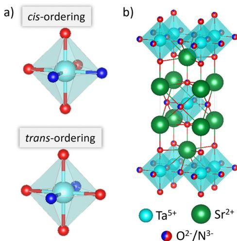
Fig. 1 (a) Anion ordering in Ta–O<sub>4</sub>N<sub>2</sub> octahedra. (b) Crystal structure of Sr<sub>2</sub>TaO<sub>3</sub>N used in this work with partial N<sup>3–</sup> occupancy of anion sites in TaON layers.
