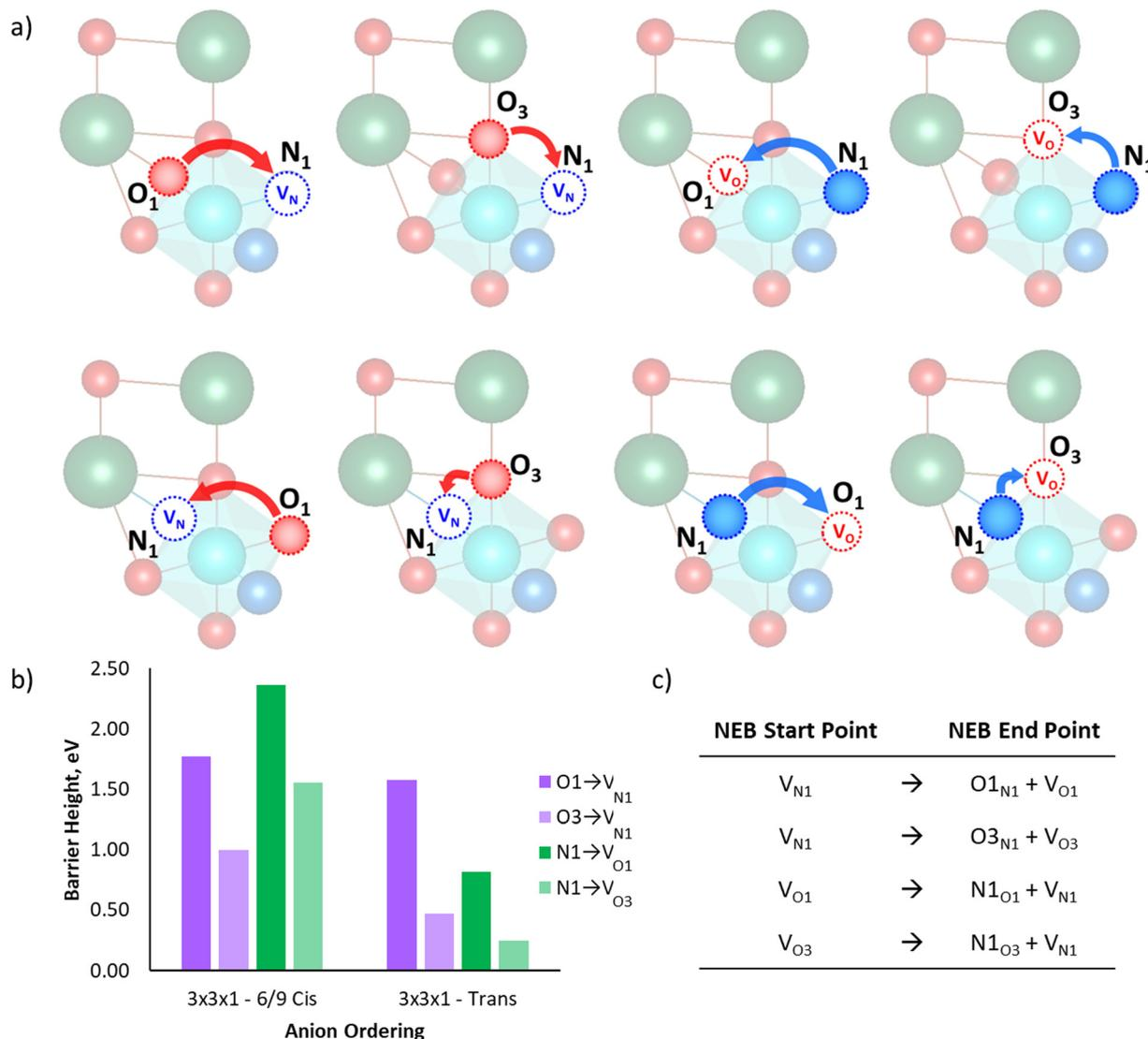
Fig. 7 (a) Anion crossing vacancy-mediated diffusion pathways around Ta-O<sub>4</sub>N<sub>2</sub> octahedra core in 6/9 *cis*- and *trans*-3 × 3 × 1 supercells and (b) PBEsol calculated NEB defect migration barrier heights for each pathway and (c) defect states at the start and end points of the NEB pathways.
