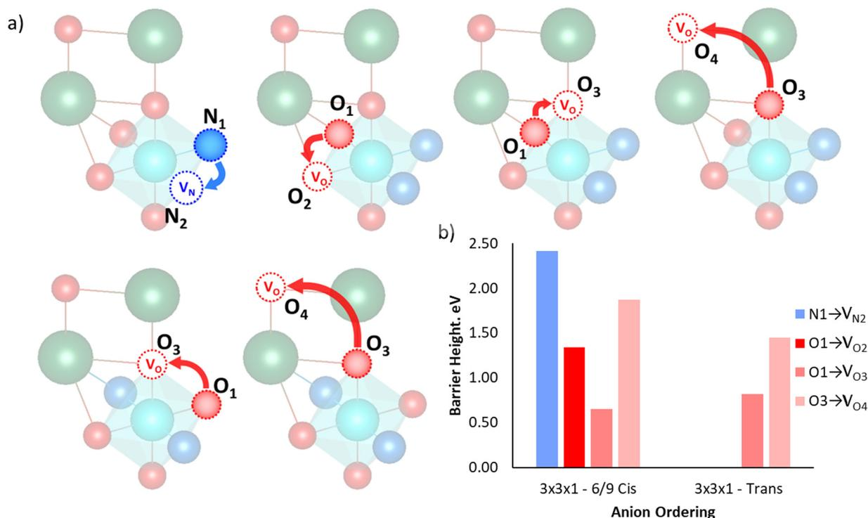
Fig. 6 (a) Native vacancy-mediated anion diffusion pathways around Ta–O<sub>4</sub>N<sub>2</sub> octahedra core in 6/9 *cis*- and *trans*- $3 \times 3 \times 1$  supercells and (b) PBEsol calculated NEB defect migration barrier heights for each pathway.
