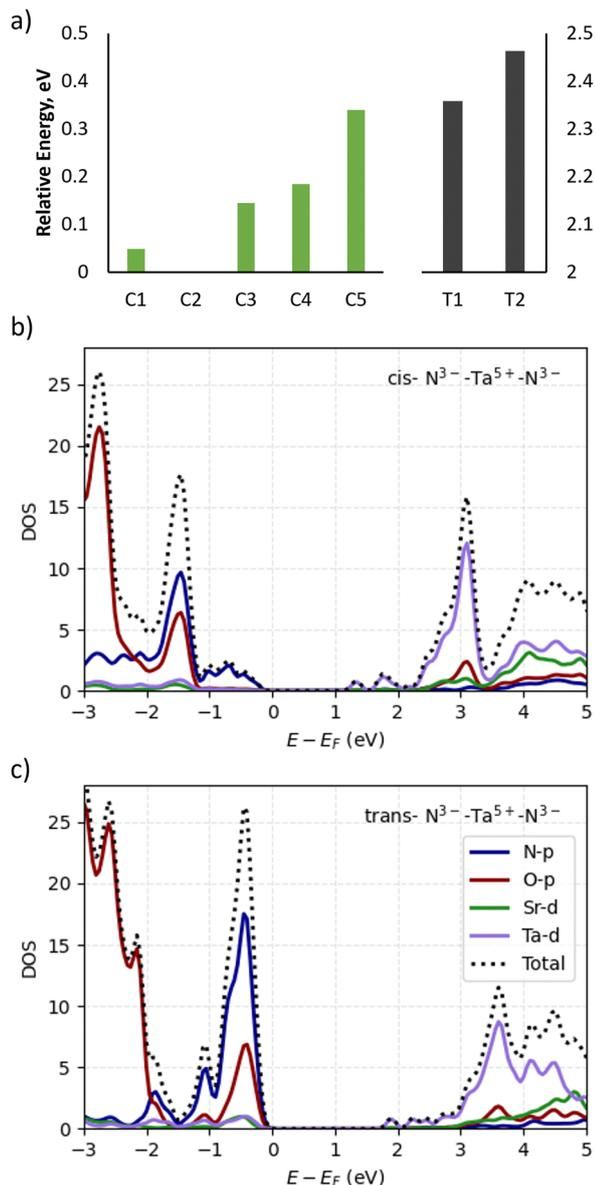
Fig. 3 (a) Relative formation energies of *cis*- and *trans*-anion orderings for the  $2 \times 2 \times 1$  Sr<sub>2</sub>TaO<sub>3</sub>N supercell. PBEsol+*U* calculated partial density of states for (b) C2 and (c) T1 anion orderings.
