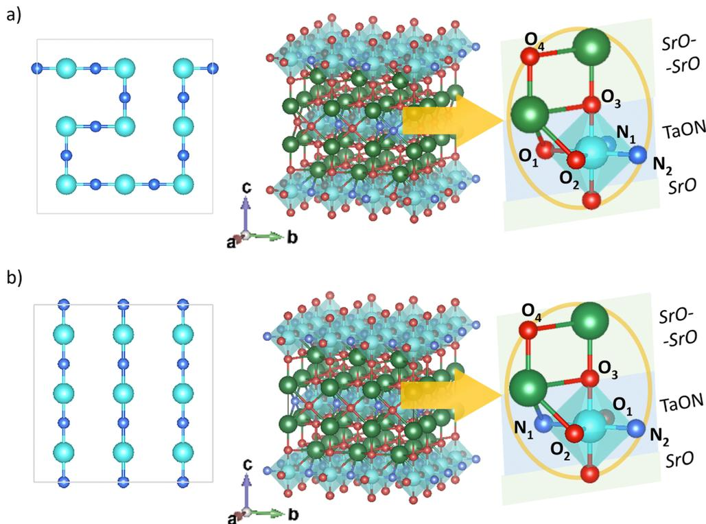
Fig. 4 (a) Representation of anion ordering constructable with the most *cis*-character;  $6/9$   $N^{3-}-Ta^{5+}-N^{3-}$  chains are *cis*- and  $3/9$  are *trans*- and (b) corresponding fully *trans*-ordering used for the  $3 \times 3 \times 1$  supercell. Insets depict anion/vacancy positions from the core of the structure used in this work, which also map to the  $2 \times 2 \times 1$  supercell.
