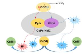
Scheme 1 The possible catalytic mechanism of Cr(vi) reduction.
