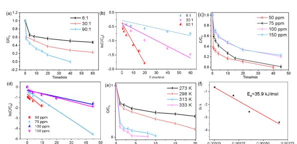
Fig. 4 (a) Effect of the molar ratio of FA and  $Cr(v_1)$  on the removal efficiency of CoPc-NMC<sub>900</sub> and (b) corresponding plots of  $ln(C_t/C_0)$  versus reaction time. (c) Effect of the concentration of  $Cr(v_1)$  on the removal efficiency of CoPc-NMC<sub>900</sub> and (d) corresponding plots of  $ln(C_t/C_0)$  versus reaction time. (e) Effect of the reaction temperature on the removal efficiency of CoPc-NMC<sub>900</sub> and (f) corresponding plots of Arrhenius.
