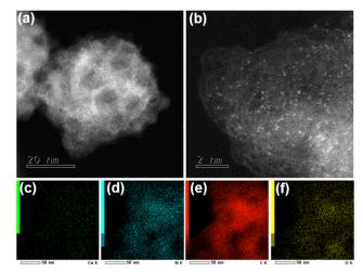
Fig. 1 (a) and (b) HAADF-STEM images and (c)–(f) corresponding elemental mappings of Co, N, C and O for 0.4% CoPc-NMC<sub>900</sub>.
