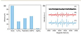
Fig. 5 (a) Control reactions performed in the presence of various scavengers. (Reaction conditions: 50 mL of Cr(vI) (50 ppm), 4.3 mmol FA, 50 mg of the catalyst, and 25 °C.) (b) EPR spectra of the (A) FA-Cr(vi) system, (B) 0.4% CoPc-NMC<sub>900</sub>/FA-Cr(vI) system with DMPO for 1 min and (C) 0.4% CoPc-NMC<sub>900</sub>/FA-Cr(vi) system with DMPO for 3 min.
