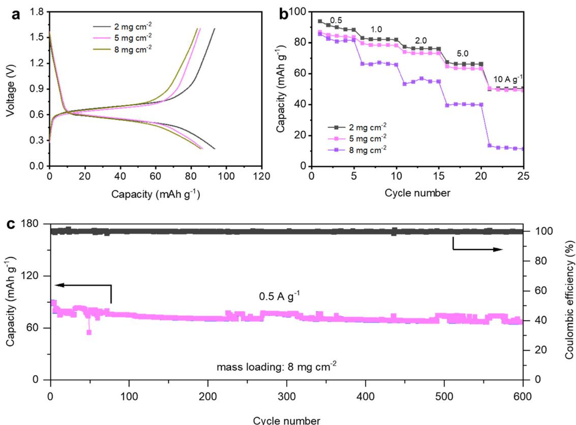
Fig. 5 (a) The discharge-charge curves of the Zn//DPPZ cell with different active mass-loading. (b) Rate capability of the Zn//DPPZ cell with various active mass-loadings. (c) Cycling performance at  $0.5\text{ A g}^{-1}$  with mass-loading of  $8\text{ mg cm}^{-2}$ .
