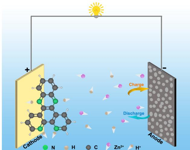
Scheme 1 Schematic illustration of the aqueous Zn//DPPZ cell.
