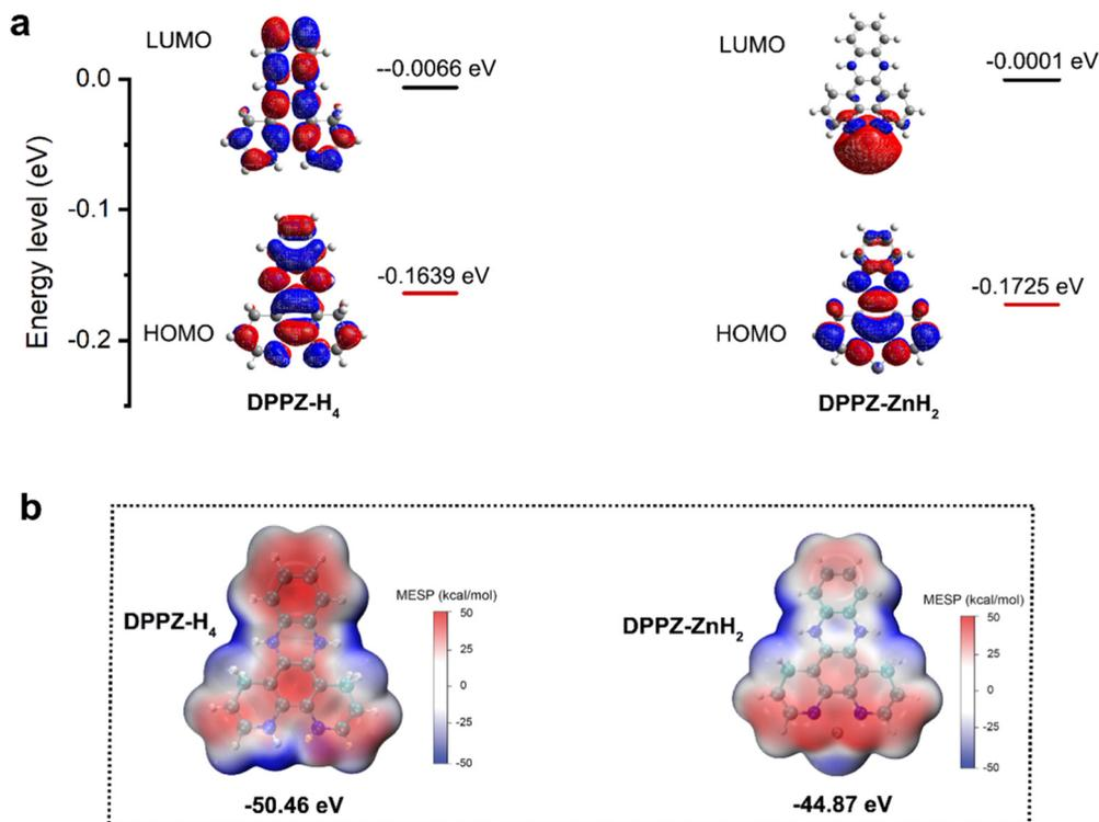
Fig. 3 (a) Optimized structures and calculated frontier molecular orbital energies of DPPZ-H<sub>4</sub> and DPPZ-ZnH<sub>2</sub> molecules. (b) Calculated MESP distributions on the van der Waals surface of DPPZ-H<sub>4</sub> and DPPZ-ZnH<sub>2</sub> molecules.
