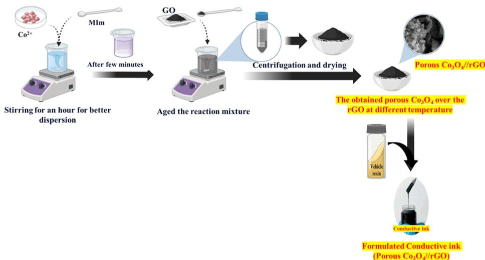
Scheme 1 Representation of the synthesis process of Co<sub>3</sub>O<sub>4</sub>/rGO and the ink formulation.
