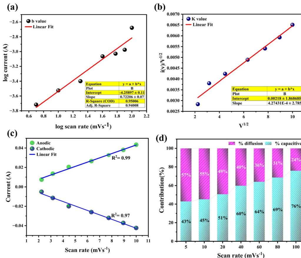
Fig. 7 (a) Logarithmic relationship between peak current and scan rate, (b) plot showing the determination of the  $k$  value, (c) determine the anodic and cathodic linear fit, (d) histogram illustrating the proportion of capacitive contributions at various scan rates.
