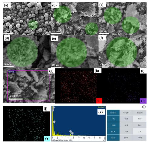
Fig. 3 SEM images showing (a) pristine Co<sub>3</sub>O<sub>4</sub>, (b) CR-1 calcined at 350 °C, (c) CR-2 calcined at 450 °C, (d) CR-3 calcined at 550 °C, (e) CR-4 calcined at 650 °C, and (f) CR-5 calcined at 750 °C. (g) EDX spectrum displaying the elemental composition of the nanocomposites. The elemental mapping shows the distribution of (h) carbon, (i) cobalt, and (j) oxygen, along with the combined elemental representation in spectra (k) and tabulated (l).
