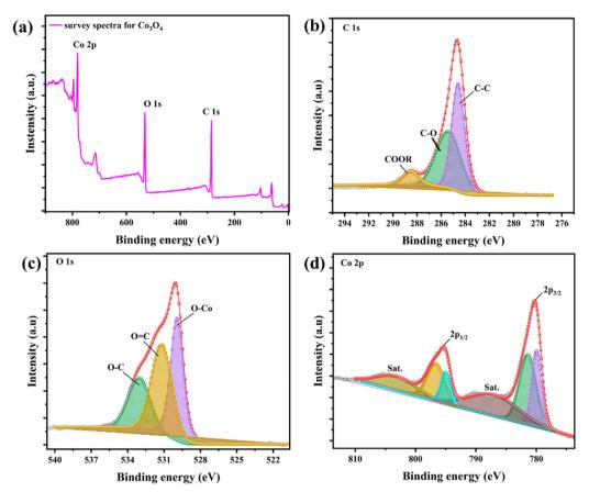
Fig. 4 Deconvoluted XPS spectra of (a) a wide scan spectrum (b) the C 1s peak (c) the O peak and (d) the Cobalt 2p peak for CR-3.
