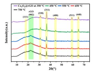
Fig. 2 Illustrates the XRD patterns of Co<sub>3</sub>O<sub>4</sub>, and rGO nanocomposite namely CR-1, CR-2, CR-3, CR-4 and CR-5
