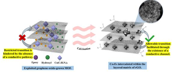
Scheme 3 Illustration of the interaction between MOF-derived Co<sub>3</sub>O<sub>4</sub> and reduced graphene oxide (rGO) during annealing
