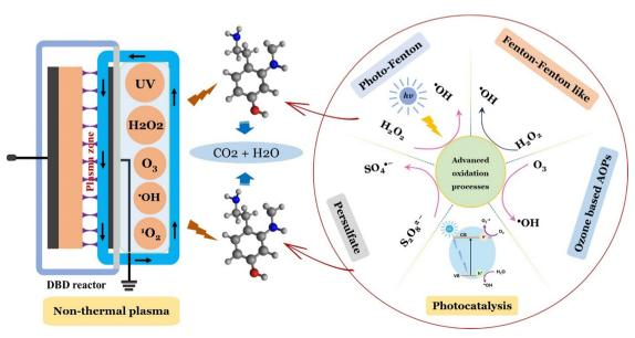
Fig. 7 Mechanism of ROS generation by various AOPs.
