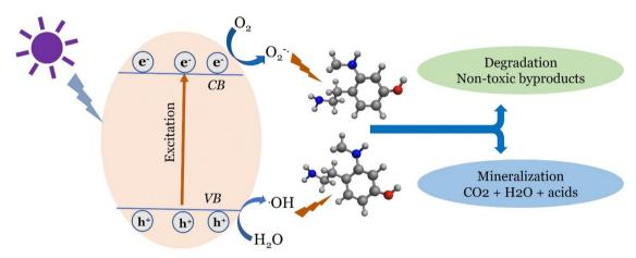
Schematic illustration of photocatalytic degradation of pharmaceuticals in water
