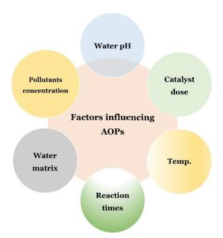
Fig. 8 Factors influencing AOP performance in pharmaceutical removal from water
