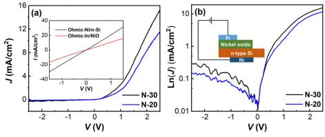
Fig. 6 Linear (a) and semi-logarithmic (b) J-V characteristics of the nickel oxide/n-Si diode. Inset of (a): I-V characteristics of Ni/n-Si and In/NiO
