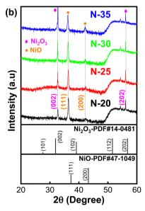
Fig. 1 X-ray diffraction (XRD) patterns of nickel oxide thin films at varying oxygen flow rates, grown on (a) glass substrate and (b) n-Si substrate.
