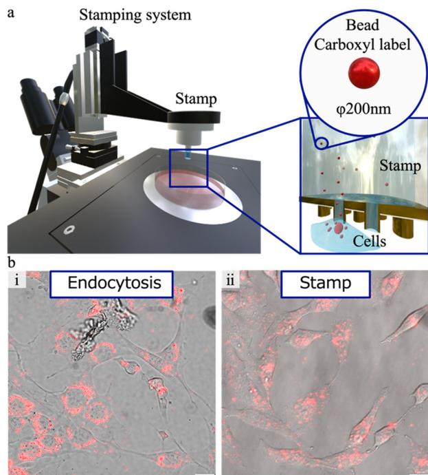
**Fig. 1** Bead delivery by the stamping system. (a) Conceptual 3D layout of the stamping system with nanotubes for the intracellular delivery of 200 nm polystyrene beads. AuNTs are highlighted. (b) Overlaid confocal bright field and fluorescence images of polystyrene beads with a diameter of 200 nm, delivered into cells by (i) endocytosis and the (ii) stamping system. The red color in (b) is fluorescence from Cy5-labeled beads. Scale bars: 20  $\mu\text{m}$ .
