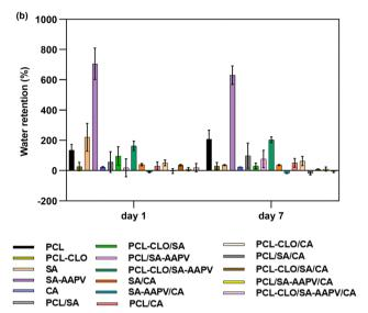
Fig. 6 Wet-spun fibers' swelling ratios (a) and water retention (b) over 7 days of incubation in PBS.
