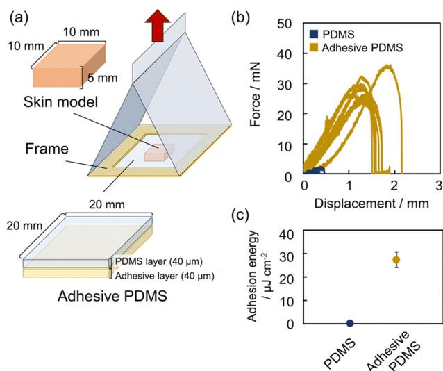
**Fig. 4** (a) The schematic image of the tack separation test of adhesive PDMS with a custom jig. (b) Results of the tack separation test and (c) calculated adhesion energy values of pristine PDMS and adhesive PDMS (PDMS = polydimethylsiloxane).
