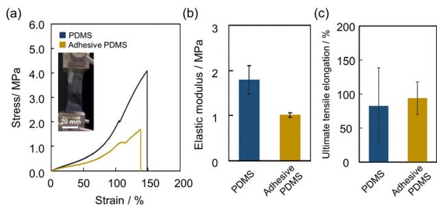
**Fig. 3** (a) Results of tensile tests on a PDMS film and an adhesive PDMS film, and the image of stretching adhesive PDMS. (b) Calculated elastic moduli and (c) ultimate tensile elongation values of each PDMS film (PDMS = polydimethylsiloxane).
