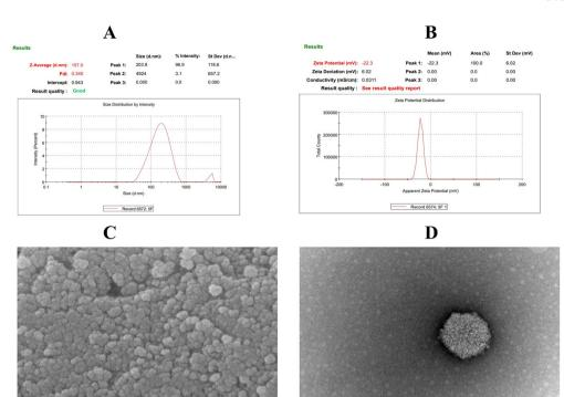
Fig. 2 Characterization of pluronic F127-decorated citric acid-capped lenvatinib-loaded porous magnetic nanoclusters (PF127/CA/LEN@pMNCs): (A) analysis of particle size; (B) measurement of zeta potential; assessment of morphology via (C) scanning electron microscopy and (D) transmission electron microscopy.
