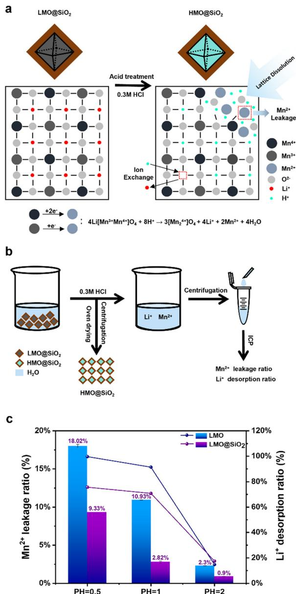
Fig. 2 (a) Schematic representation of the mechanism and dissolution process from LMO@SiO<sub>2</sub> to HMO@SiO<sub>2</sub> acid treatment. (b) Schematic diagram of Li<sup>+</sup> and Mn<sup>2+</sup> adsorption-desorption processes and ICP characterization of treated solutions. (c) Li<sup>+</sup> desorption and Mn<sup>2+</sup> leakage ratio of LMO and LMO@SiO<sub>2</sub> at different pH values.
