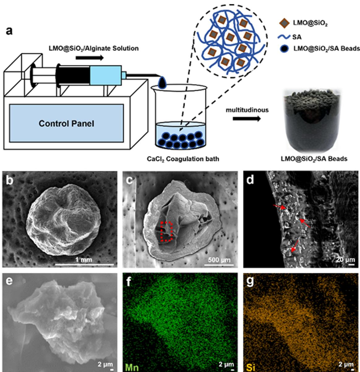
**Fig. 3** (a) Schematic of granulation of LMO@SiO<sub>2</sub> and actual images of LMO@SiO<sub>2</sub>/SA beads. (b)–(d) SEM characterization of whole, cross-sectional, and internal venation of LMO@SiO<sub>2</sub>/SA beads. (e)–(g) High magnified SEM image and the corresponding EDS characterization of Mn and O elements of the embedded LMO@SiO<sub>2</sub> powder.
