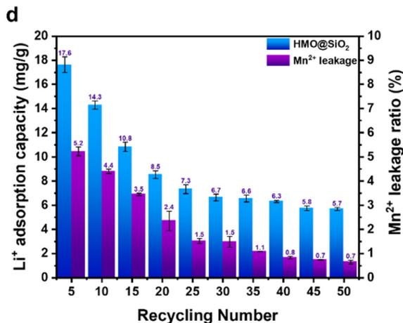
Fig. 5 (a) and (b) Schematic and actual images of the continuous flow adsorption–desorption cycle system. (c) Photograph of Da Qaidam Salt Lake in Qinghai Province. (d) ICP analysis of the Li<sup>+</sup> adsorption capacity and Mn<sup>2+</sup> dissolution ratio over 50 cycles.
