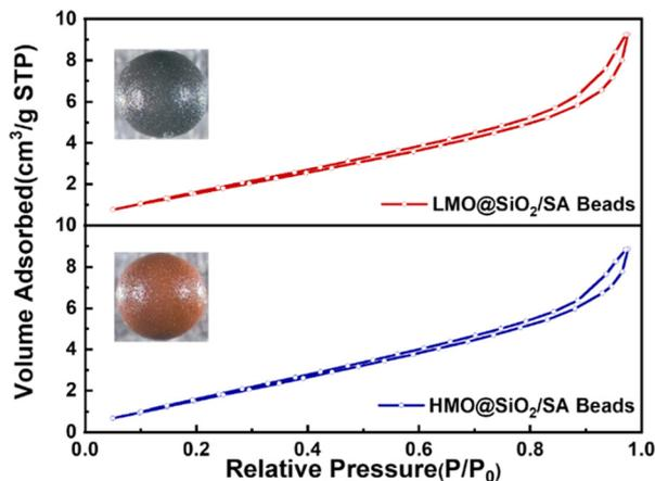
Fig. 4 BET analysis of the adsorption pore volume for LMO@SiO<sub>2</sub>/SA beads and HMO@SiO<sub>2</sub>/SA beads. Insets are the corresponding single beads before (LMO) and after (HMO) acid treatment.
