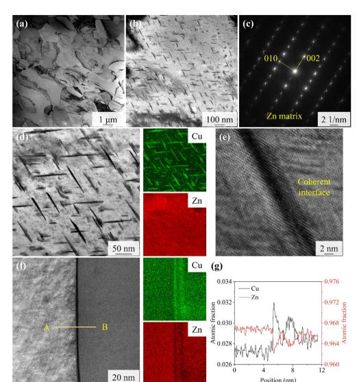
Fig. 3 TEM images of the Zn-0.4Cu alloy: (a) grain regions. (b) Plate-shaped precipitates. (c) SAED image. (d) Precipitates and the corresponding element distributions. (e) HR-TEM image of precipitates. (f) Grain boundary and the corresponding element distributions. (g) Atomic fractions of Zn and Cu.
