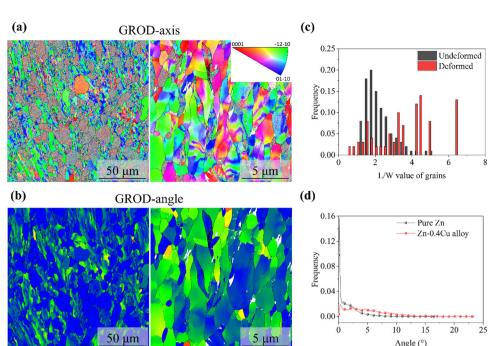
Fig. 11 Microstructural analysis of a deformed specimen: (a) GROD axis. (b) GROD angle. (c) Ratio of the length and width of grains in the Zn-0.4Cu alloy before and after fracture. (d) FROD angle distributions of the fractured pure Zn and Zn-0.4Cu alloy.
