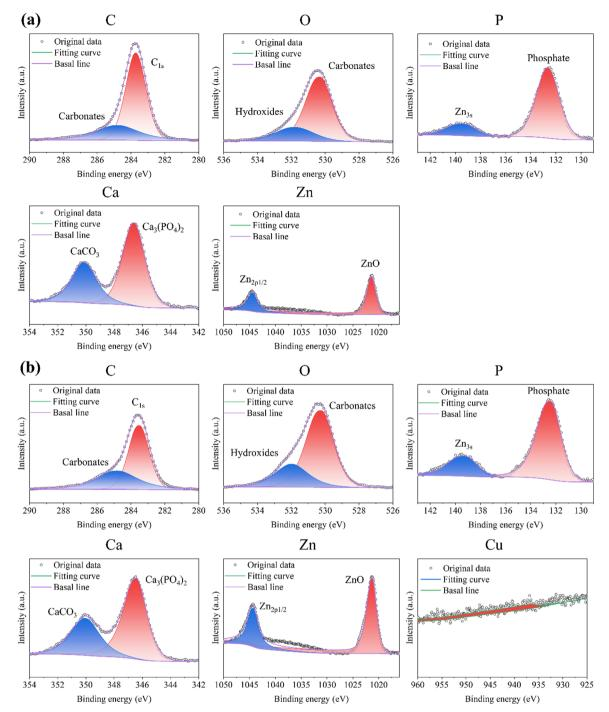
Fig. 7 Narrow spectra of the corrosion products: (a) pure Zn. (b) Zn-0.4Cu.
