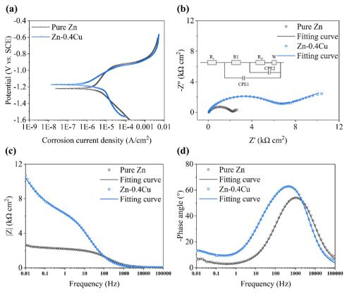
Fig. 5 Electrochemical behavior of the samples: (a) PDP curves. (b) Nyquist plots and fitting curves (inert image shows the fitting circuit). (c) |Z| and (d) -phase angle vs. frequency.
