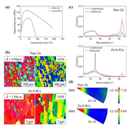
Mechanical behaviors of the samples: (a) typical tensile curves. (b) IPF and GOS mappings. (c) Misorientations. (d) IPF textures
