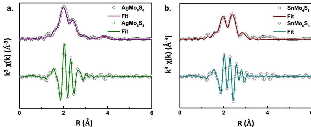
Fig. 4 Mo K-edge FT-EXAFS data (circle) and fits (lines) with components of the FT  $k^3\chi(k)$  in non-phase corrected magnitude on the top and in real on the bottom for (a)  $\text{AgMo}_6\text{S}_8$  and (b)  $\text{SnMo}_6\text{S}_8$ .
