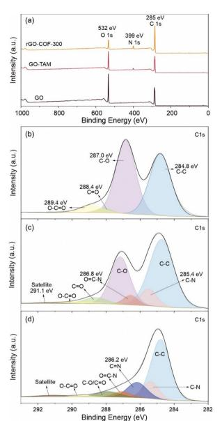
**Fig. 2** (a) Wide scanning XPS spectra of the GO, GO–TAM and rGO–COF-300. High-resolution C 1s spectra of (b) GO, (c) GO–TAM and (d) rGO–COF-300. The C 1s XPS spectrum of GO exhibits five peaks at about 284.8, 287.0, 288.4, 289.4 and 291.1 eV, which corresponds to C–C, C–O (including hydroxyl, epoxy, *etc.*), C—O, O–C—O and C satellite bonds, respectively. 43,44
