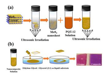
Fig. 1 (a) Synthesis mechanism of PQT-12/MoS<sub>2</sub> nanocomposite. (b) Schematic diagram of thin film formation by floating film transfer method and optical image of prepared films over glass substrate.
