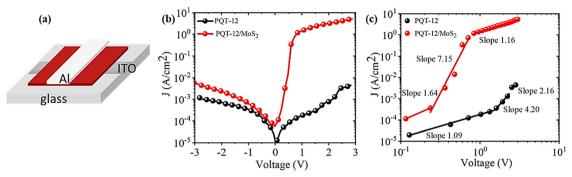
Fig. 7 (a) Schematic representation of the fabricated SBD devices. (b) J-V characteristics of the ITO/PQT-12/Al and ITO/PQT-12-MoS<sub>2</sub>/Al devices. (c) log J versus log V plot for Au/PQT-12/Al, and Au/PQT-12-MoS<sub>2</sub>/Al.
