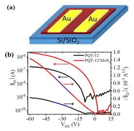
Fig. 6 (a) Schematic representation of the fabricated OFET devices. (b) Transfer characteristics of pristine PQT-12 and PQT-12/MoS<sub>2</sub> filmbased OFETs.
