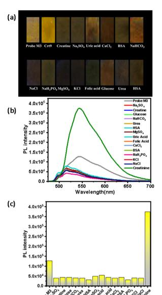
Fig. 4 (a) Photographs of M3-impregnated filter paper strips under a UV lamp (365 nm) after dipping into different aqueous solutions of urine components; (b) corresponding PL spectra (excitation wavelength of 370 nm); (c) bar graph showing the PL intensity for the corresponding solutions.
