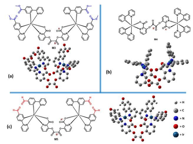
Fig. 7 Basic unit structure and the optimized geometry using DFT via Gaussian 16 with the LanL2DZ basis set and PBEPBE functional: (a) for M3, (b) for M4, and (c) for M5 with the labeled characteristic bonds, i.e., picolinate carbonyl (as A, A', and A") and oxalate carbonyls as (B, B', and B").
