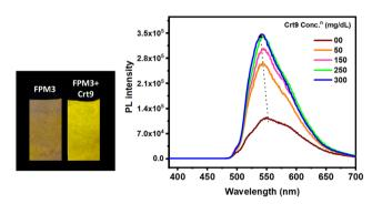
Fig. 3 Photographs of the filter paper impregnated with M3 (FP-M3) before and after being dipped in aq. creatinine (Crt9) (300 dL) under a UV lamp (365 nm) and their corresponding PL intensity plot for FP-M3 at an excitation wavelength of 370 nm, showing a steady variation of the PL intensity with gradually increasing concentrations of aq. creatinine (Crt9) (dotted arrow indicates the blue shift with emission enhancement).
