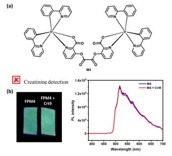
Fig. 5 (a) Chemical structure for the synthesized dinuclear iridium(III) complex **M4** and (b) luminescent response on a filter paper strip impregnated with **M4** (*i.e.*, FPM4) under a UV lamp (365 nm) with the corresponding PL intensity spectra (excitation at  $\lambda_{\rm exc}=370$  nm).
