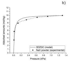
Fig. 6 Comparison between the model CO<sub>2</sub> (a) and water vapour (b) adsorption isotherms of the NaX-rich, 3D-printed zeolite-geopolymer composite and the corresponding experimental isotherms of pristine NaX powders at 298.15 K.
