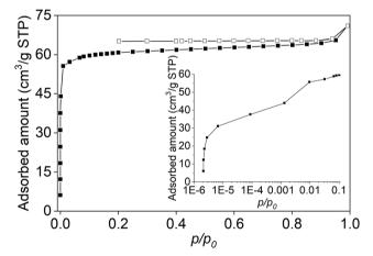
Fig. 4 N<sub>2</sub> adsorption (solid symbols)/desorption (open symbols) isotherm at 77 K of the NaX-rich, 3D-printed zeolite-geopolymer composite.
