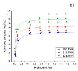
Fig. 5 CO<sub>2</sub> (a) and water vapour (b) adsorption isotherms (triplicate measurements) of the NaX-rich, 3D-printed zeolite-geopolymer composite at 298.15, 318.15 and 338.15 K. Continuous lines: best fitting Toth model isotherms.
