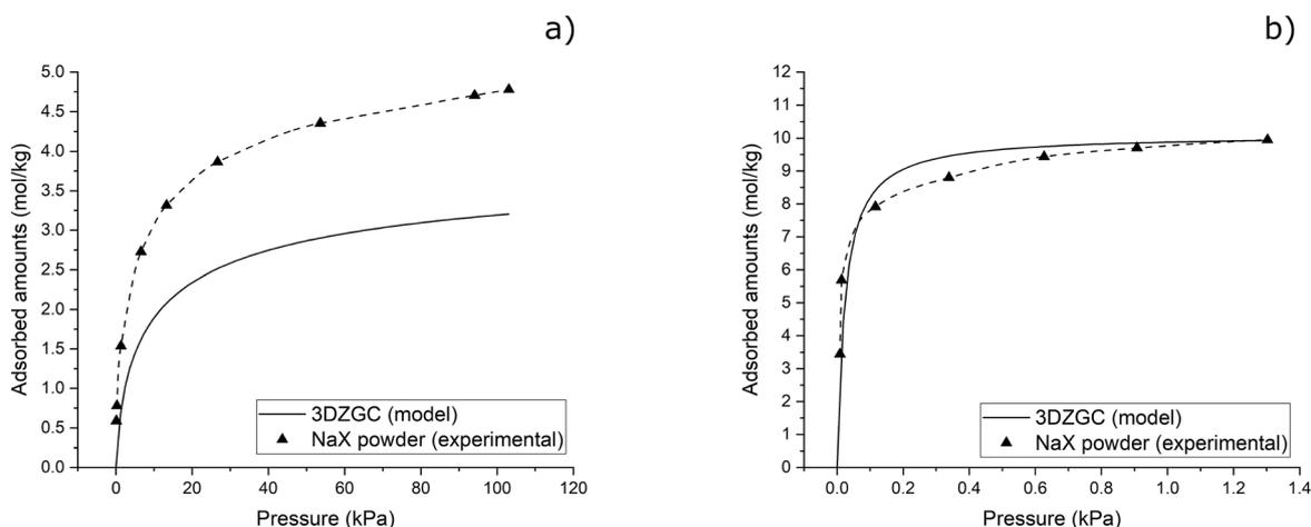
Fig. 6 Comparison between the model CO<sub>2</sub> (a) and water vapour (b) adsorption isotherms of the NaX-rich, 3D-printed zeolite–geopolymer composite and the corresponding experimental isotherms of pristine NaX powders at 298.15 K.
