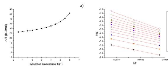
Fig. 7 Isosteric heat of water vapour adsorption on the NaX-rich, 3D-printed zeolite-geopolymer composite (a) and the corresponding isostere plot (b).
