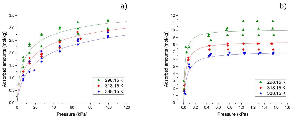
Fig. 5 CO<sub>2</sub> (a) and water vapour (b) adsorption isotherms (triplicate measurements) of the NaX-rich, 3D-printed zeolite-geopolymer composite at 298.15, 318.15 and 338.15 K. Continuous lines: best fitting Toth model isotherms.
