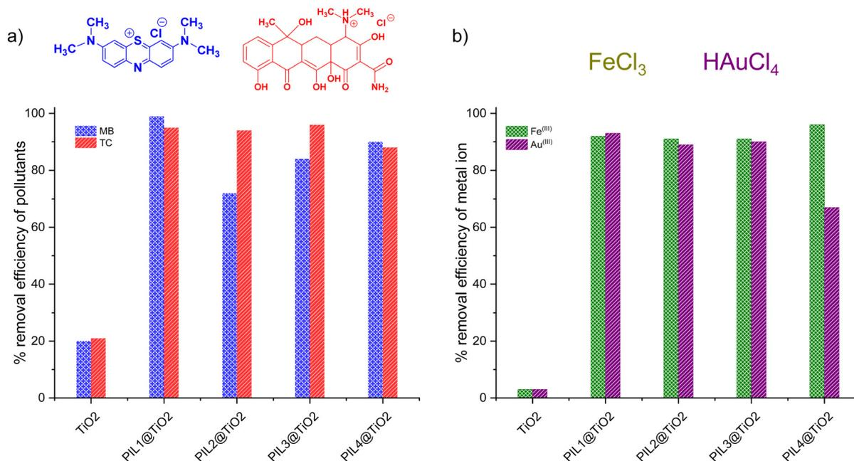
Fig. 5 Removal of (a) methylene blue (MB) and tetracycline (TC), and (b) removal of  $\text{Fe}^{(\text{III})}$  and  $\text{Au}^{(\text{III})}$  using  $\text{TiO}_2$  and  $\text{PIL}_n\text{@TiO}_2$  materials.
