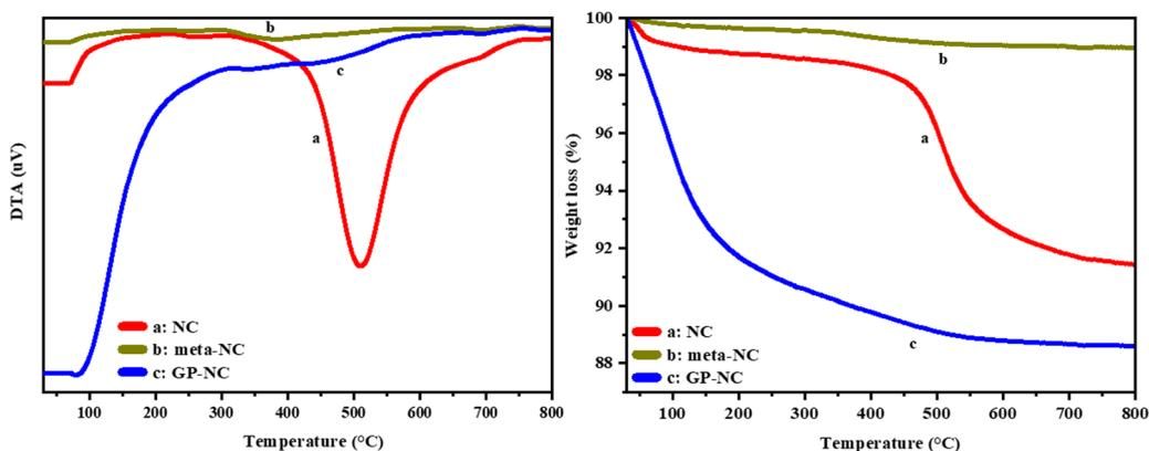
Fig. 5 TGA/DA curves of NC, *meta*-NC, and GP-NC.
