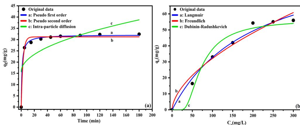
Fig. 9 (a) adsorption kinetics, (b) adsorption isotherms.
