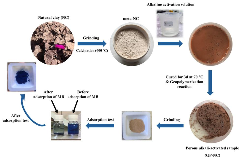
Fig. 2 Schematic preparation of the porous alkali-activated material.
