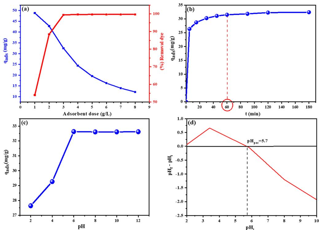
Fig. 8 (a) Effect of adsorbent dose; (c) effect of contact time; effect of pH on the adsorption of MB on GP-NC; (d) point zero charge ( $\text{pH}_{\text{pzc}}$ ).
