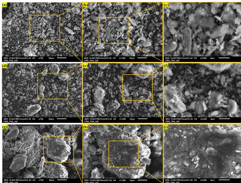
Fig. 6 SEM and TEM micrographs of *meta*-NC (a–c), GP-NC (d–f), and GP-NC@BM (g–i).
