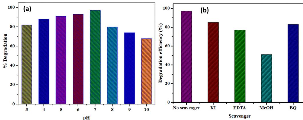
Fig. 10 (a) Effect of pH value of the solution on MG dye degradation, and (b) effect of scavengers on the degradation efficiency of MG dye over the Co@BFO nanocomposite.
