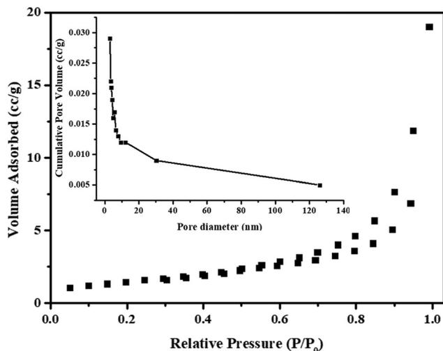
Fig. 7  $N_2$  adsorption-desorption spectra of the Co@BFO-III nanocomposite.
