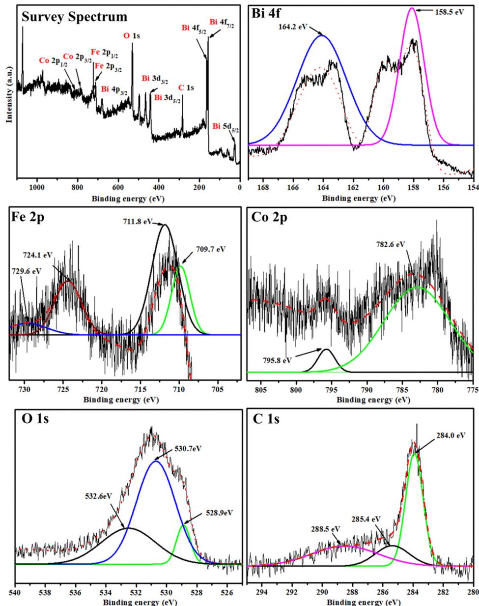
Fig. 6 XPS analysis of the Co@BFO-III nanocomposite.
