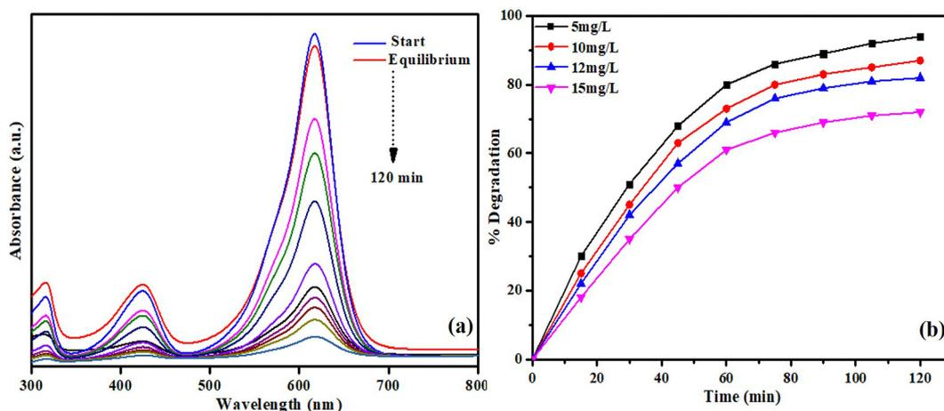
Fig. 8 (a) UV-Visible absorbance spectrum of MG dye degradation vs. time and (b) percentage degradation of MG dye at different initial concentrations (5, 10, 12, and 15  $mg L^{-1}$ ) over 120 minutes.
