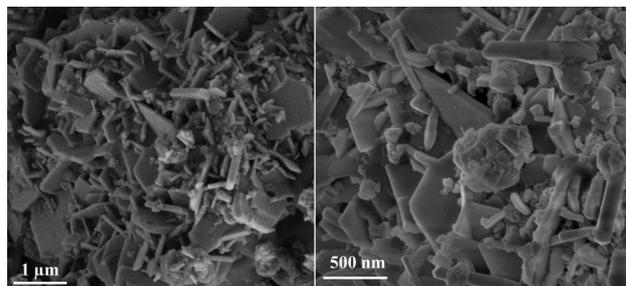
Fig. 2 FESEM micrographs of the Co@BFO-III nanocomposite.
