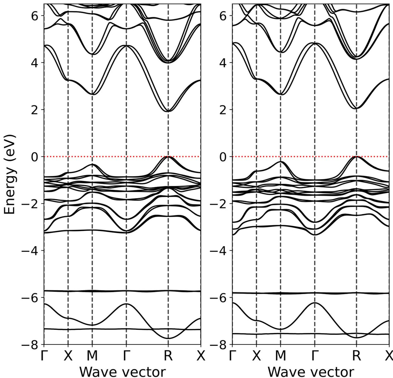
Fig. 1 Band structure of pseudocubic MAPbI<sub>2</sub>Br (left hand side) and MAPbIBr<sub>2</sub> (right hand side) calculated at the level of AK13/GAM theory. Zero eV is at the valence band maximum.
