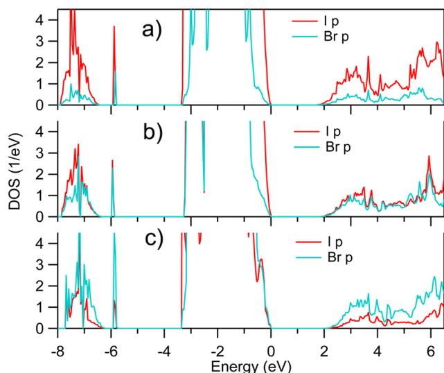
Fig. 3 Zoom onto unoccupied I p and Br p densities of states of pseudocubic  $\text{MAPb}(\text{I}_{1-x}\text{Br}_x)_3$  calculated for (a)  $x = 0.25$ , (b)  $x = 0.50$ , and (c)  $x = 0.75$ , respectively.
