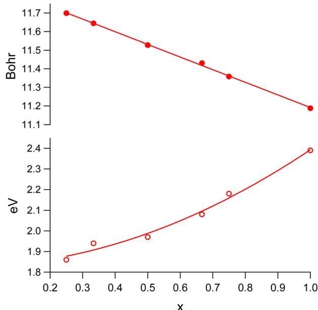
Fig. 4 The optimized lattice parameter (solid markers) and band gap size (open markers) of  $\text{MAPb}(\text{I}_{1-x}\text{Br}_x)_3$  in the cubic structure region.
