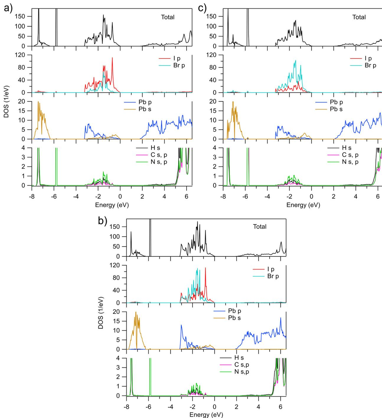
Fig. 2 Total and partial densities of states of pseudocubic MAPb(I<sub>1–*x*</sub>Br<sub>*x*</sub>)<sub>3</sub> calculated for (a) *x* = 0.25, (b) *x* = 0.50, and (c) *x* = 0.75, respectively. Zero eV is at the valence band maximum.
