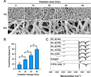
Fig. 2 Electrospun PCL/collagen composite scaffolds following gammaray irradiation: (A) SEM images, (B) degrees of crosslinking, (C) FT-IR spectra of scaffolds subjected to radiation doses ranging from 15 to 45 kGy.
