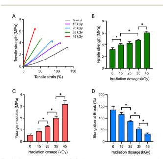
**Fig. 4** Tensile properties of PCL/collagen composite scaffolds following gamma-ray irradiation: (A) stress–strain curve, (B) ultimate tensile strength, (C) Young's modulus, and (D) elongation at break (%).
