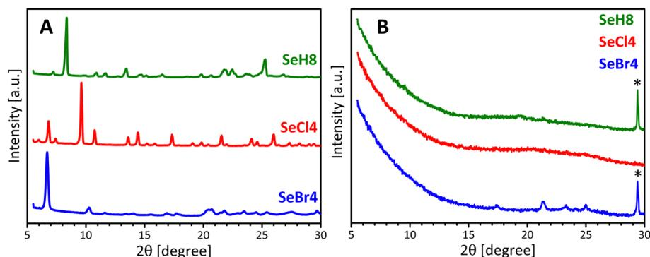
Fig. 3 (A) XRD patterns of **SeH<sub>8</sub>**, **SeCl<sub>4</sub>** and **SeBr<sub>4</sub>**; (B) *ex situ* XRD patterns of electrodes **SeH<sub>8</sub>**, **SeCl<sub>4</sub>** and **SeBr<sub>4</sub>** cycled in a lithium-ion cell for 50 cycles (\*peaks of Al foil).
