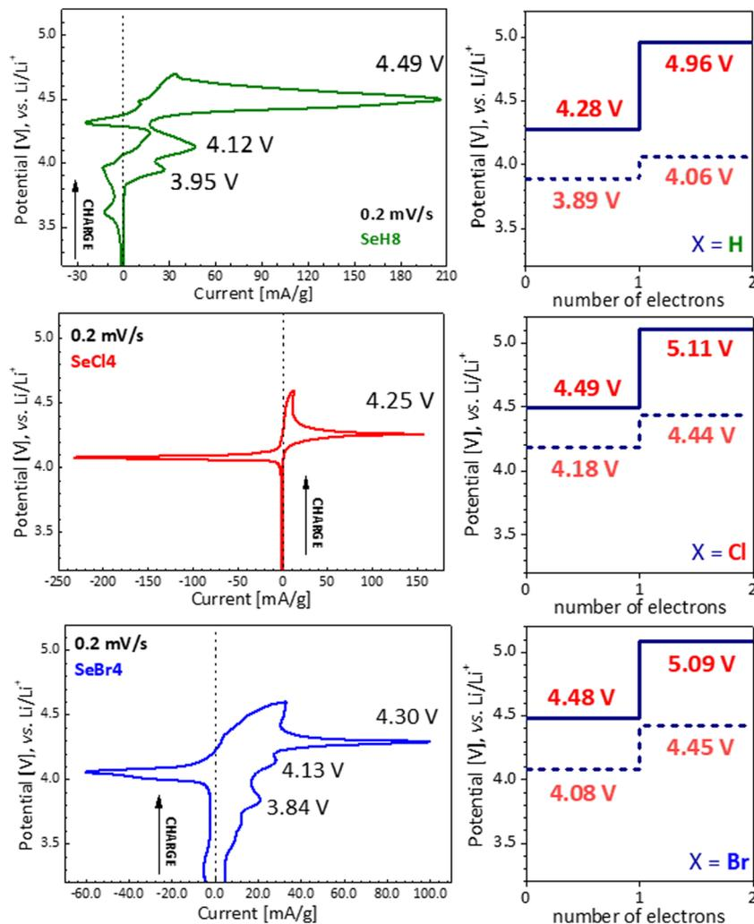
Fig. 7 (left) Cycling voltammograms of **SeH8**, **SeCl4** and **SeBr4** started with an anodic scan. (right) Theoretically calculated potentials for single and double oxidation of molecules without and in the presence of counterion TFSI<sup>-</sup> (full and dotted lines, respectively).
