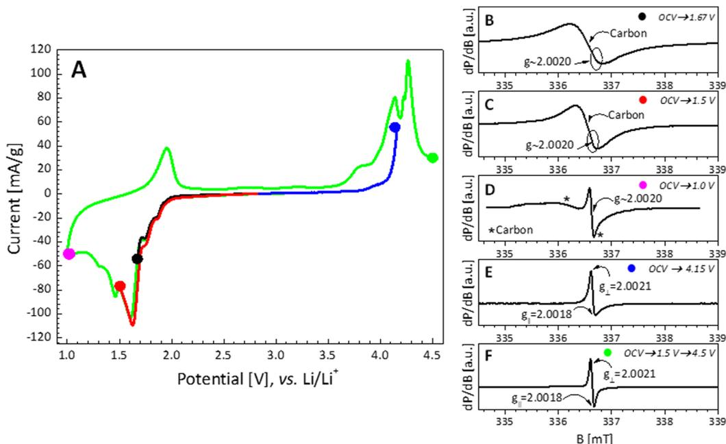
Fig. 8 CV curves (A) and the respective *ex situ* EPR analysis of **SeCl<sub>4</sub>** electrodes: after the first cathodic scan up to 1.67 V (B; black), then to 1.5 V (C; red) and to 1.0 V (D; magenta); after the first anodic scan to 4.15 V (E; blue), and after the cycle starting with cathodic scan to 1.0 V, followed with an anodic scan to 4.5 V (F; green). All spectra are recorded at  $T = 100$  K.
