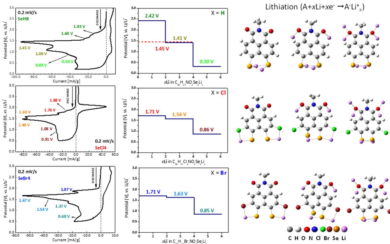
Fig. 6 Cycling voltammograms of **SeH8**, **SeCl4** and **SeBr4** started with a cathodic scan, theoretically calculated potentials and optimized geometries of the *peri*-diselenolo derivatives with different number of Li ions.
