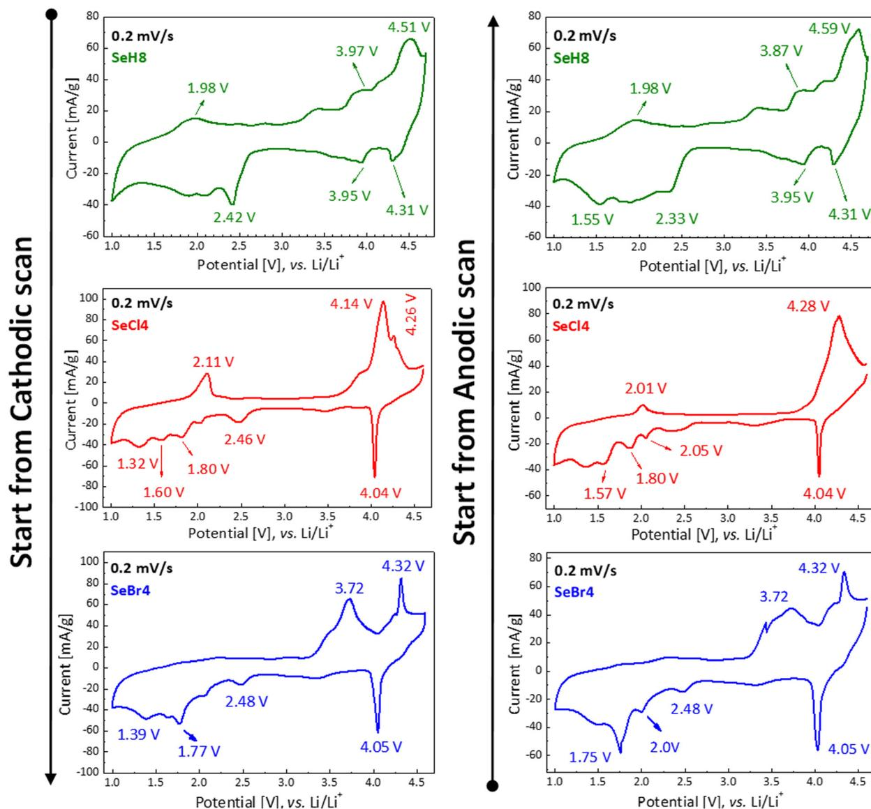
Fig. 9 CV curves after the fifth scan for **SeH8** (green lines), **SeCl4** (red lines), and **SeBr4** (blue lines) used as electrodes in three-electrode cells started with a cathodic and anodic scan, respectively.
