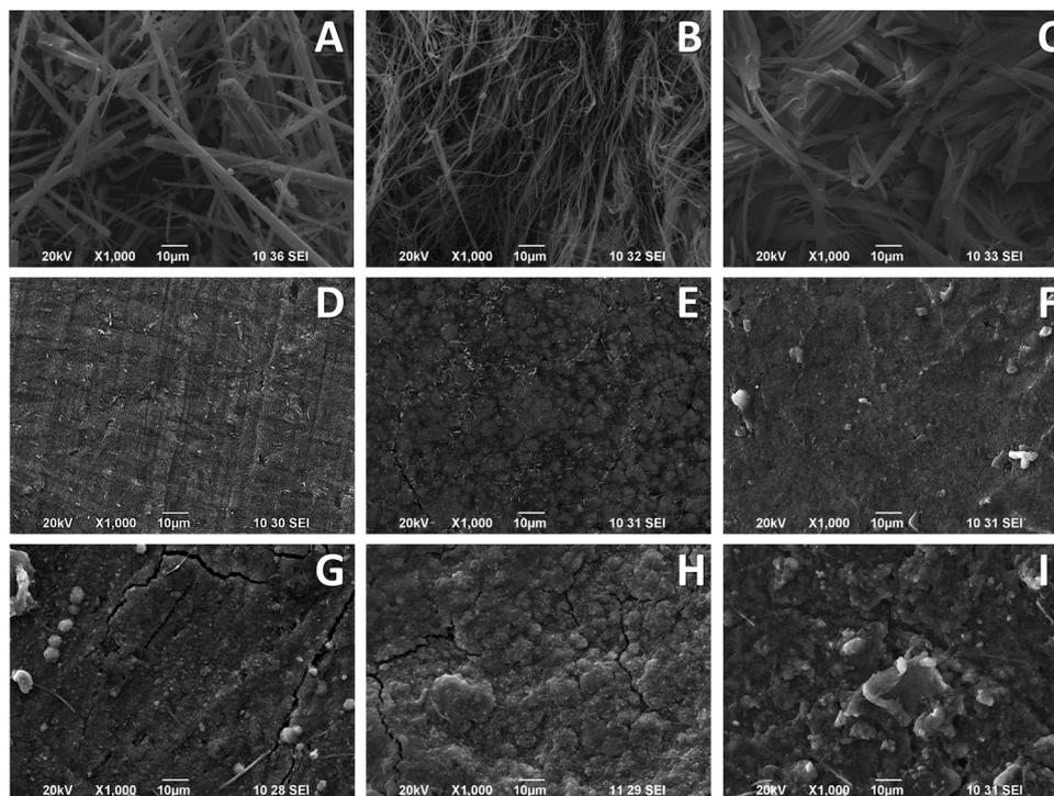
Fig. 2 SEM images of pristine **SeCl<sub>4</sub>**, **SeBr<sub>4</sub>** and **SeH<sub>8</sub>** (A)–(C) and corresponding bare electrodes (D)–(F). The *ex situ* images of electrodes cycled for 50 times (G)–(I) in LiTFSI:Py<sub>1.3</sub>FSI electrolyte. The fibres correspond to the GF/A separator.
