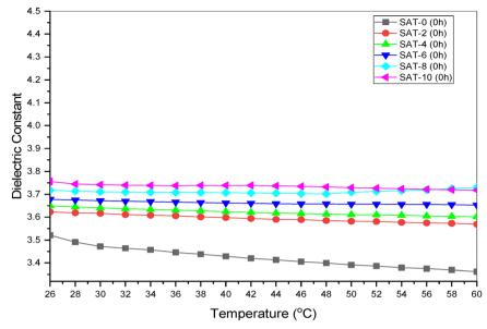
Fig. 10 Dielectric constant of unaged samples (Varying Temperature).
