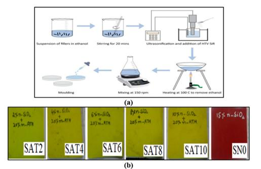
Fig. 2 Sample preparation (a), preparation process (b), and images of the prepared samples
