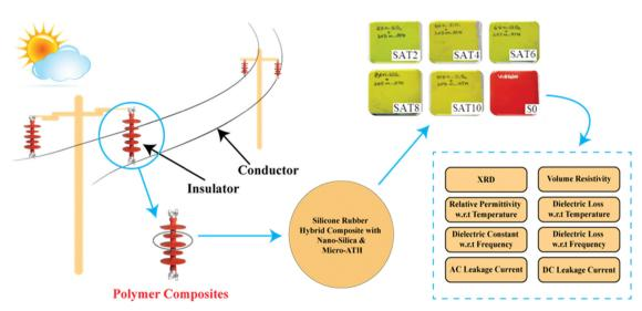
Fig. 1 Schematic description of conducted work.
