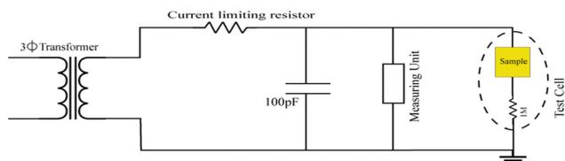
Fig. 4 Setup for measurement of AC leakage current.
