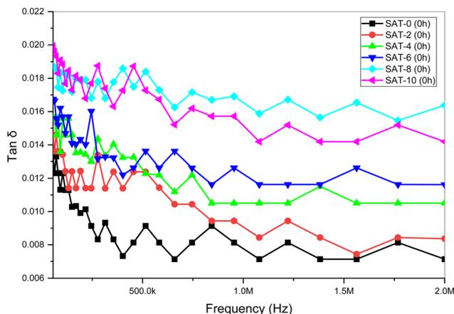
Fig. 18  $\tan \delta$  of the unaged samples.
