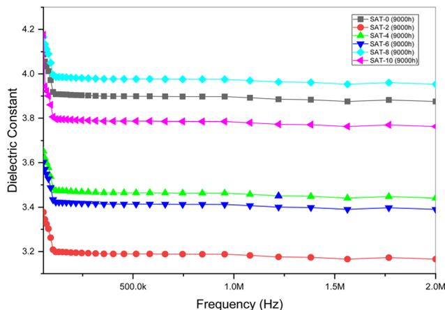
Fig. 17 Dielectric constant of the aged samples.
