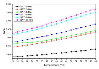
Fig. 12  $\tan \delta$  of the unaged samples.
