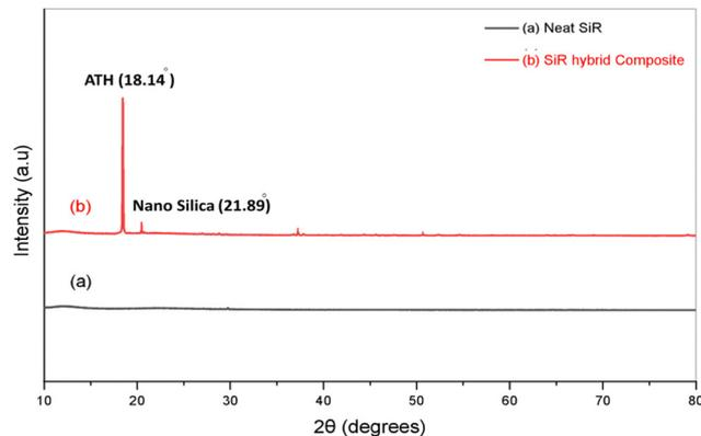
Fig. 5 XRD pattern of (a) neat HTV silicone rubber and (b) silicone rubber hybrid composite.
