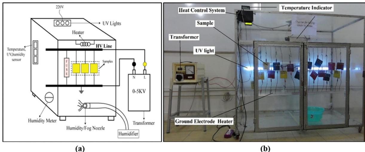
Fig. 3 Multi stressed aging chamber (a), schematic diagram (b) and actual picture.
