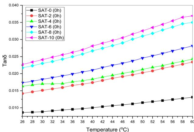
Fig. 12  $\tan \delta$  of the unaged samples.
