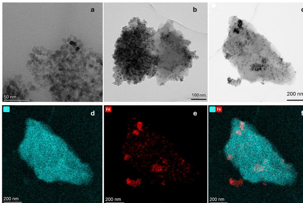
Fig. 2 HRTEM pictures of bare  $\text{Fe}_3\text{O}_4$  and MAC platforms. (a) bare  $\text{Fe}_3\text{O}_4$ ; (b) and (c) MAC; (d) EDX mapping analysis of C element of MAC particles; (e) EDX mapping analysis of Fe element of MAC particles; (f) EDX mapping analysis of overlapped C and Fe elements of magnetic carbon activated nanoplatforms.
