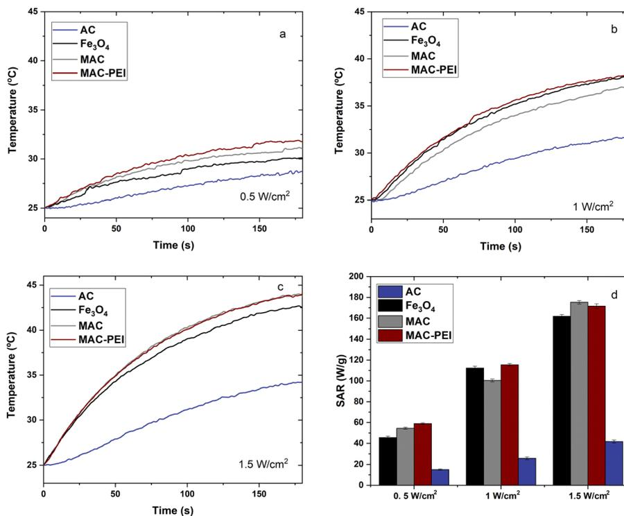
Fig. 6 Temperature increases for PTT therapy, at a power irradiation of  $0.5 \text{ W cm}^{-2}$  (a),  $1 \text{ W cm}^{-2}$  (b), and  $1.5 \text{ W cm}^{-2}$  (c), using  $100 \mu\text{L}$  of sample at  $5 \text{ mg mL}^{-1}$ . Determination of the SAR obtained (d).
