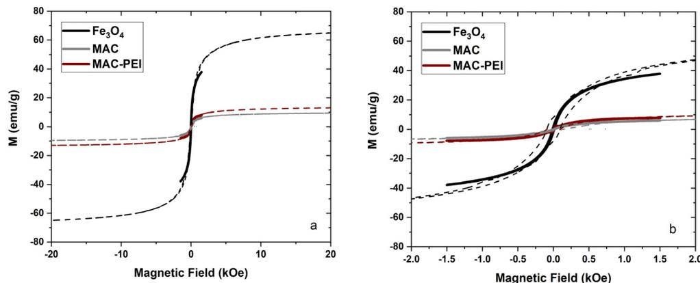
Fig. 5 Magnetic characterization of the obtained MAC nanoporous particles. (a) Magnetization curves of the bare  $\text{Fe}_3\text{O}_4$ , MAC and PEI coated particles using VSM (dotted lines) and AC magnetometry (solid lines); (b) low-field detail of the plots in (a). Hysteresis cycles carried out at 300 K.
