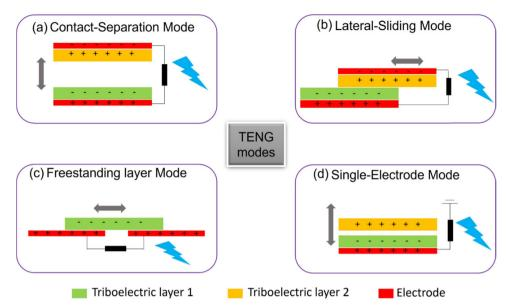
Fig. 10 Four operating modes of TENGs.
