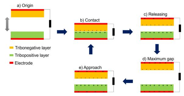
Fig. 11 Working principle of vertical contact-separation mode.
