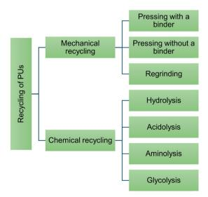
Fig. 9 Recycling methods for PU materials.
