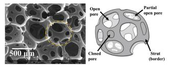
Fig. 8 Schematic representation of the morphology of FPU foam, reproduced from ref. 107 with permission from Elsevier, copyright 2024
